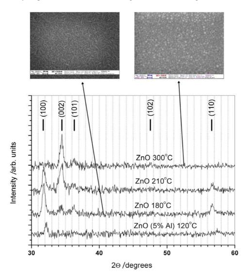
A relationship between crystalline morphology vs. temperature and aluminium incorporation was established. The above figure summarizes the XRD characterization results of our samples. Two characteristic SEM micrographs are also presented, reflecting the morphology for the two preferential crystalline orientations in the ZnO layers. These are the (100), when the c axis of the ZnO unit cell is parallel with the substrate, and the (002), where the c axis is normal to the surface [7].
