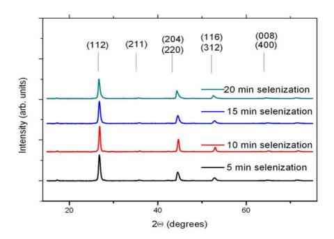
XPS results obtained on the CIGS layers post-selenized at 500°C for different durations. Only the diffraction peaks of the chalcopyrite structure are present, no oxides or selenides are visible, whatsoever [8].
