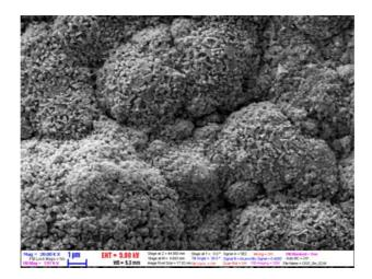
SEM micrograph of the flash evaporated and post selenized (500°C for 15 min) CIGS layer. Note the cauliflower-like morphology [8].
