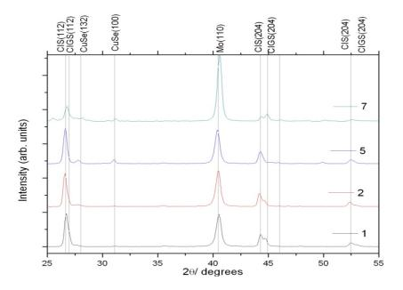
Comparison of the XRD spectra of differently processed CIGS layers (samples 1, 2, 5 and 7). Summary of the phases identified by XRD in the samples 5-8. selenized with constant vapour pressure.
