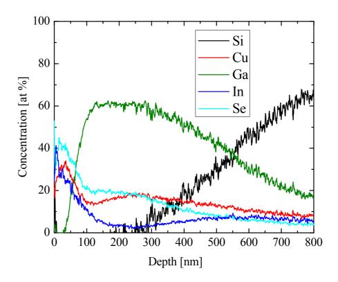
SNMS depth profiles of the CIGS layer selenized at 500° for 15 minutes. In this concentration plot no Ga accumulation was observable at the bottom of the CIGS layer, the depth of which is indicated by the increase of the Si concentration originating from the glass substrate [8].
