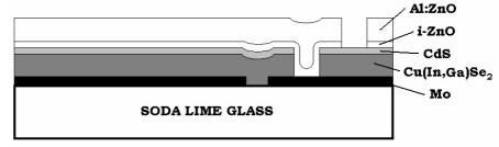
"The subject of the present materials research project is the active region of the structure, the p-type CIGS layer (grey) and the n-type buffer layer (here CdS) on top of it. The corresponding band diagram is shown below.
