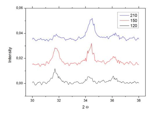
The intrinsic ZnO samples above were deposited at three different substrate temperatures (120°C, 150°C, 210°C) and their spectra can be considered typical The most intensive XRD peaks can be found at  $2\Theta = 31,77^{\circ}$  the (100), at  $2\Theta = 34,42^{\circ}$  the (002), and at  $2\Theta = 36,25^{\circ}$  the (101), respectively [5]. We could state that:
