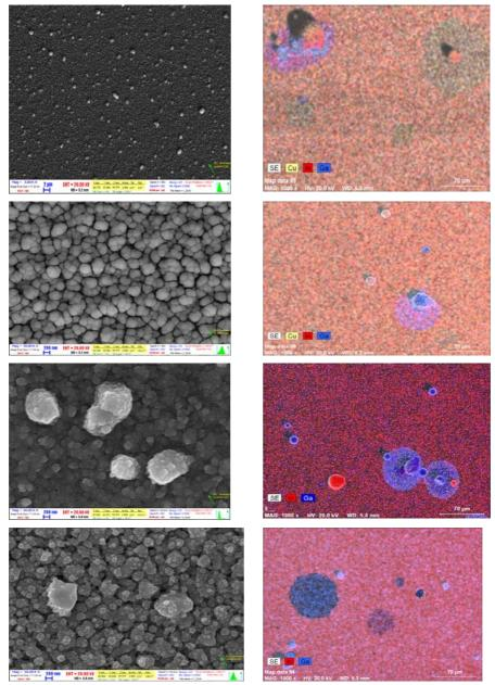
SEM micrographs (left) at 5000x in (a) and 50000x magnification (c,e,g) and element maps of the evaporated precursors (right) for sample 1, 2, 3 and 4 in the respective rows [9].
