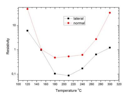
Specific resistance (in  $X10^{-2}$  cm<sup>-3</sup>) of the 2 at% Al-doped sample parallel and perpendicular to the layer surface vs. deposition temperature for the determination of the optimum growth conditions [7, 27].
