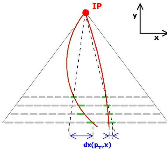
Figure 2: The magnetic field ( $B=0.5$  T) of the ALICE detector diverts the charged particles inside the magnet. The radius of the path is large for small momentum and small for large momentum. The 4-layer structure can identify the radius and can work as a threshold trigger. The simulations indicate an optimal threshold of 9-10 GeV/c.
