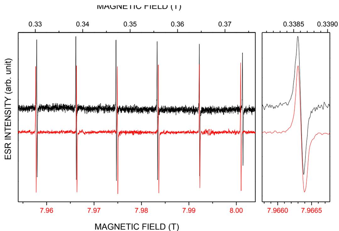
Fig. 4. Comparison of the room temperature spectra of 1mg Mn:MgO powder (Mn concentration 1.58 ppm) recorded in a commercial Bruker Elexsys E500 at 9.4 GHz (upper curve) and in our home-built spectrometer at 222.4 GHz (lower curve). Close-up on the right shows that the line width is 0.1 mT in both measurements thus there is no instrumental broadening. The spectral resolution is 25 times larger at high frequencies.
