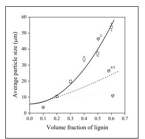
**Fig. 2** Comparison of the reliability of published theories and their range of validity for LDPE/lignin blends. Models: .......... Fortelný and Kovář [7]; \_\_\_\_\_\_ Huneault et al. [8]; \_\_\_\_\_\_ this project.
