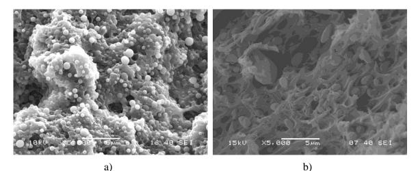
**Fig. 1** Structure of ionomer/lignin blends prepared with lignins produced by dissimilar technologies. a) Kraft lignin, b) lignosulfonate. The blends contained 20 vol% lignin.
