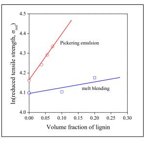
**Fig. 4** Effect of the preparation technique on the load bearing capacity of lignin in *PLA*/lignin blends.
