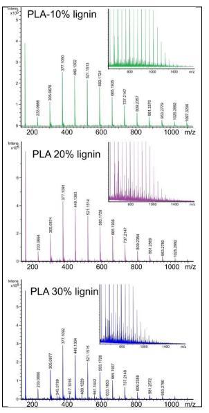
**Fig. 7** Maldi spectra of lignin-g-PLA copolymers; lignin content (10-30 wt%) increases from top to bottom.
