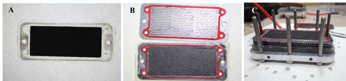
Fig. 13. (A) Electrode with an active area of 15 cm 2 on the membrane, (B) MEAs are sealed with silicone gaskets and (C) stacking.
