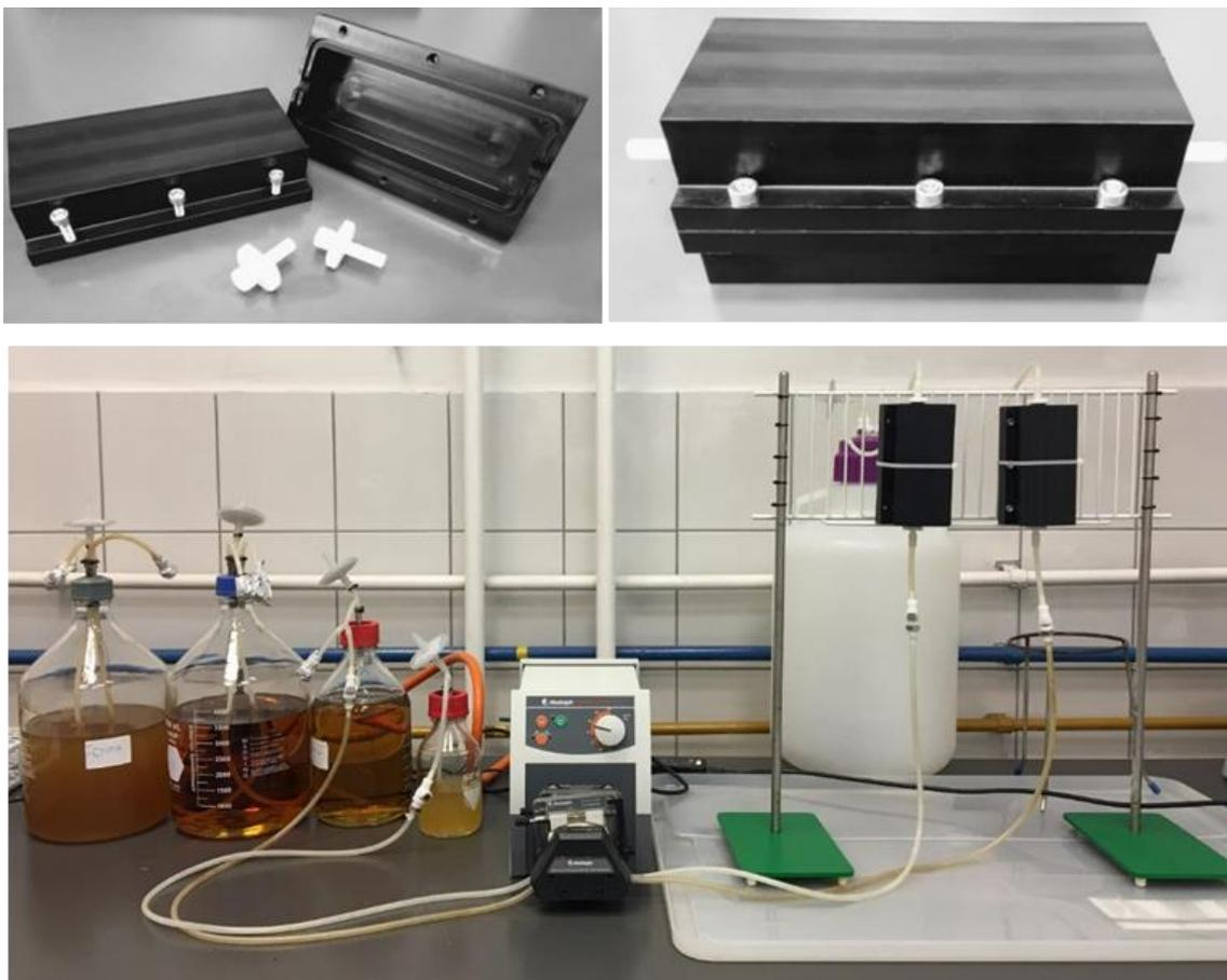
**Figure 7.** Lab-scale bio-cementing model system. Molds used for the bio-cementing of the porous matrix are shown in the upper part of the figure.
