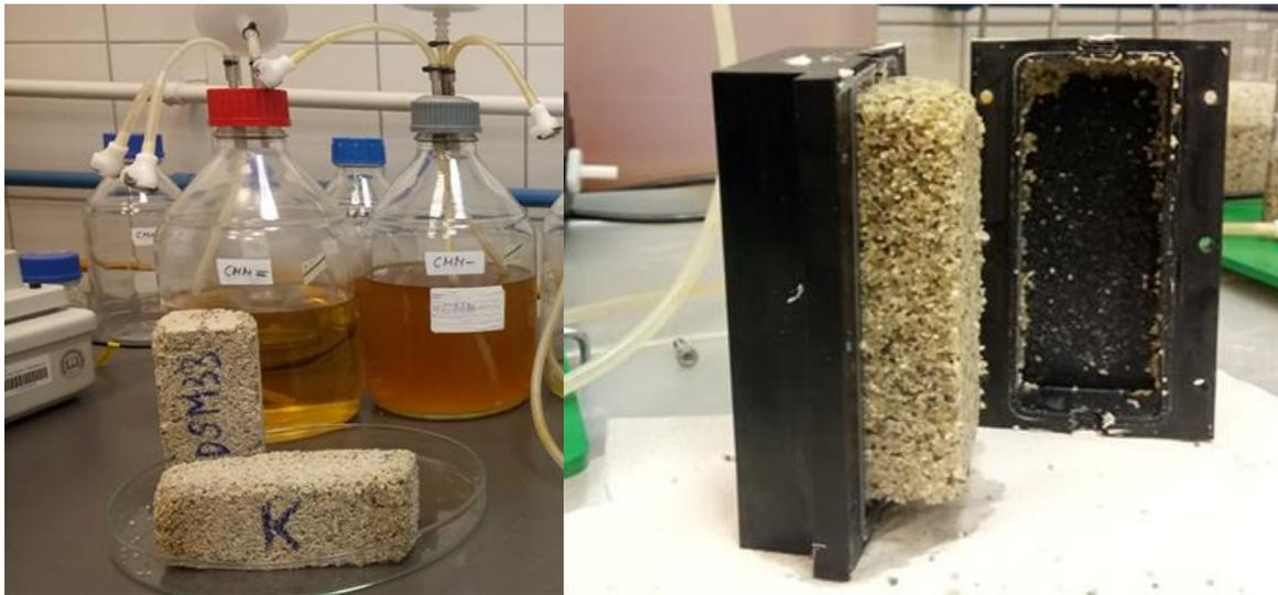
**Figure 8.** The bio-cemented porous matrix obtained by using the engineered consortium (K) or the *S. pasteurii* DSM 33 alone (DSM 33).
