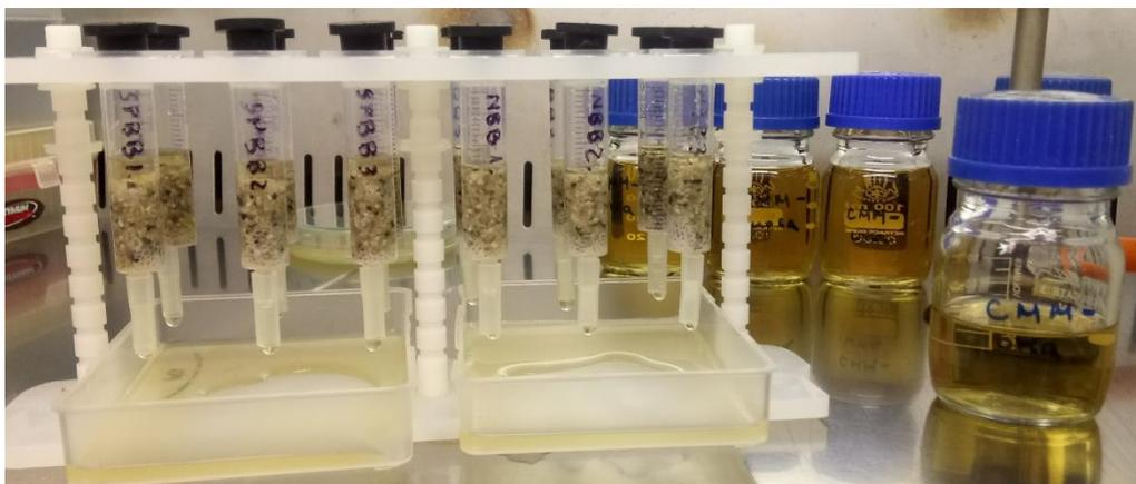
**Figure 9.** Lab-scale mineral-biobarrier systems used for investigating the reactive nature of the bio-cemented porous matrix.
