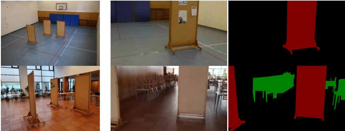
Figure 1. Test area and sample images from the drone camera. The first row shows the first test site, the gym of the University. The second row shows the second test site, the dining hall of the University. The left column is an overview of the environment with the obstacles. The middle column is the image from the drone camera, and the right column is the annotated image showing the object masks. The red mask is the display panel, and the green mask is the table with chairs.
