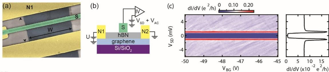
Figure 5: Tunnel spectroscopy measurements. a) Device outline. Blue is graphene, green is the SC tunnel contact, whereas yellow contacts are made from normal metal. b) Measurement scheme. c) Differential conductance (without heating bias) as a function of bias and gate voltage. By performing and averaging over the gate voltage to reduce UCF, the DOS of the SC is recovered.
