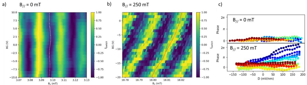
Figure 3: Large  $\varphi_0$  phase for WSe<sub>2</sub>/BLG/WSe<sub>2</sub>. Switching current (modulation) as a function of back-gate and external magnetic field for 0T (a) and for 250mT (b). c) Extracted phases as a function of displacement field for different densities (colours). A large gate tuneable phase is visible in finite magnetic fields.
