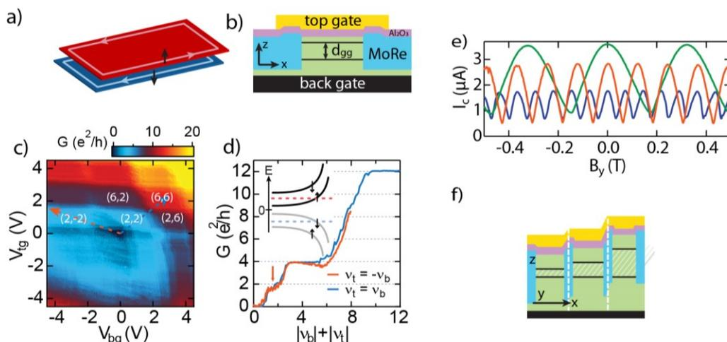
Figure 4: Measurements on the double layer setup. a) Sketch of artificial QSHE. b) Device sketch. c) Conductance as a function of the top and bottom gate voltage at 5T. d) Cuts from c) shown by the dashed
