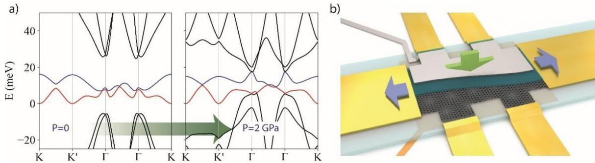
Figure 6: a) Band structure of twisted double bilayer graphene (with twist angle of 1.07) at ambient and large pressures. A strong modification of the bandstructure is observed. b) Artistic view of a device, with the green arrow showing the hydrostatic pressure.
