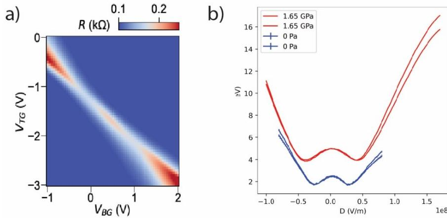
Figure 2: a) Differential resistance as a function of top and bottom gate voltages in a WSe<sub>2</sub>/BLG/WSe<sub>2</sub> heterostructure. The bright colours show gaps at the charge neutrality point. At large voltages the displacement field opens up a gap, whereas at low displacement fields the SOC opens a gap. b) Extracted gaps as function of displacement field for ambient and high pressure. The curves show a clear increase of the gaps around zero displacement field.
