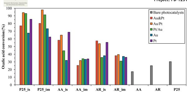
Figure 3 Oxalic acid degradation performances after 1 h of the obtained nanocomposites under UV light. All of the composites showed higher photocatalytic activity than their corresponding base photocatalyst. Results after 2 h were omitted as each composite degraded the oxalic acid totally.
