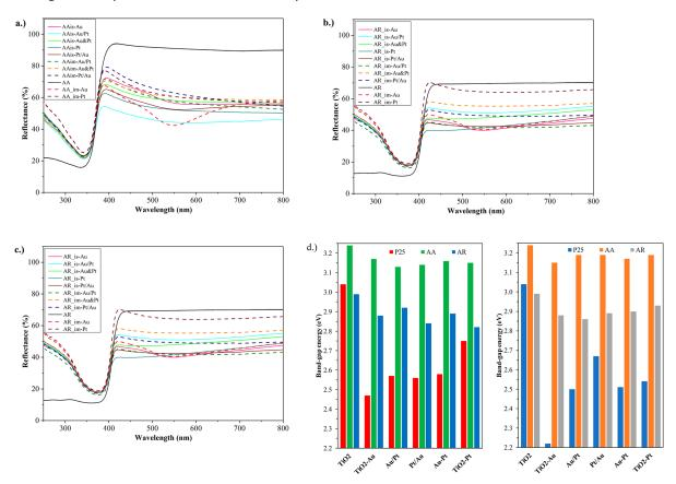
Figure 1: Influence of the noble metals on the optical properties of three commercial titania (a - AA; b - AR; c - P25; d, band gap energy comparison using the in situ sample series-left and impregnation series-right). The influence was significant when P25 was the base photocatalyst, while in the other cases, no changes were observed in their spectrum.
