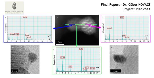
Figure 2: STEM-HAADF (b) micrograph, HR-TEM (d, f) images, and EDS spectra (a, c, and e) of P25imp-Au/Pt sample, showing the presence of both Au and Pt. No core-shell particles and no alloys were detected, just nanoparticles, which show Pt and/or Au presence.
