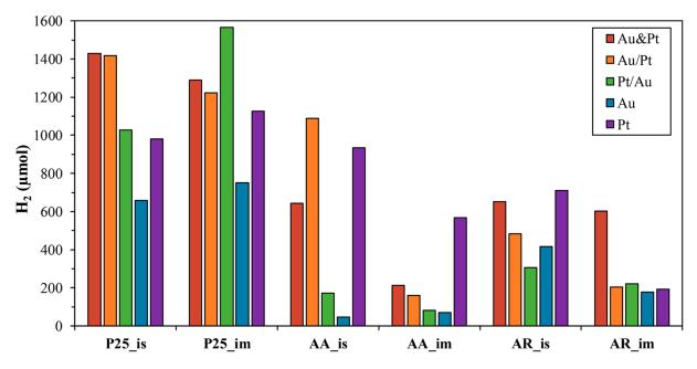
*Figure 5 Photocatalytic H2 production capacities of the used nanocomposites. The bare photocatalysts were not shown, as they do not produce hydrogen under these experimental conditions*
