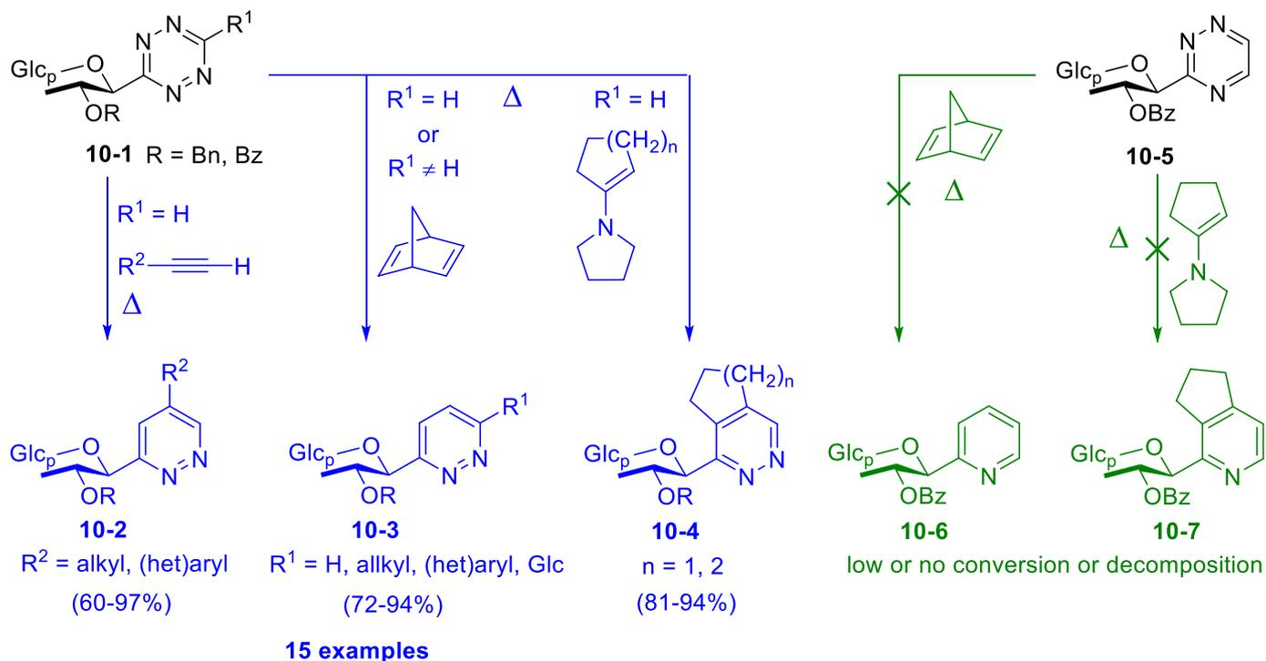
**Scheme 10.** Experiments towards 3-( $\beta$ -D-glucopyranosyl)pyridazines and 2-( $\beta$ -D-glucopyranosyl)pyridines by IEDDA reactions
