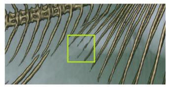
Prefiltered triquadratic B-spline interpolation using our fast evaluation scheme: 6.69 fps.
