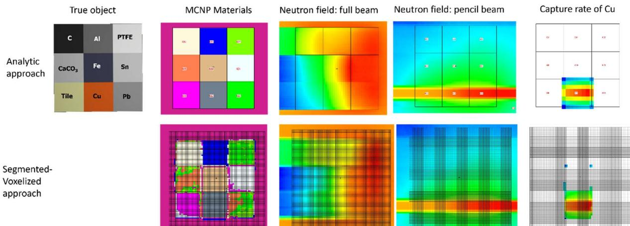
Figure 1. The simulated neutron field and capture rate of a  $3 \times 3 \times 3$  structured cube assembly
