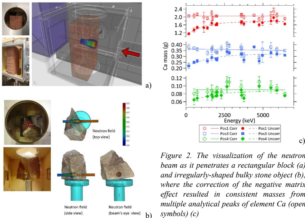
Figure 2. The visualization of the neutron beam as it penetrates a rectangular block (a) and irregularly-shaped bulky stone object (b), where the correction of the negative matrix effect resulted in consistent masses from multiple analytical peaks of element Ca (open symbols) (c)
