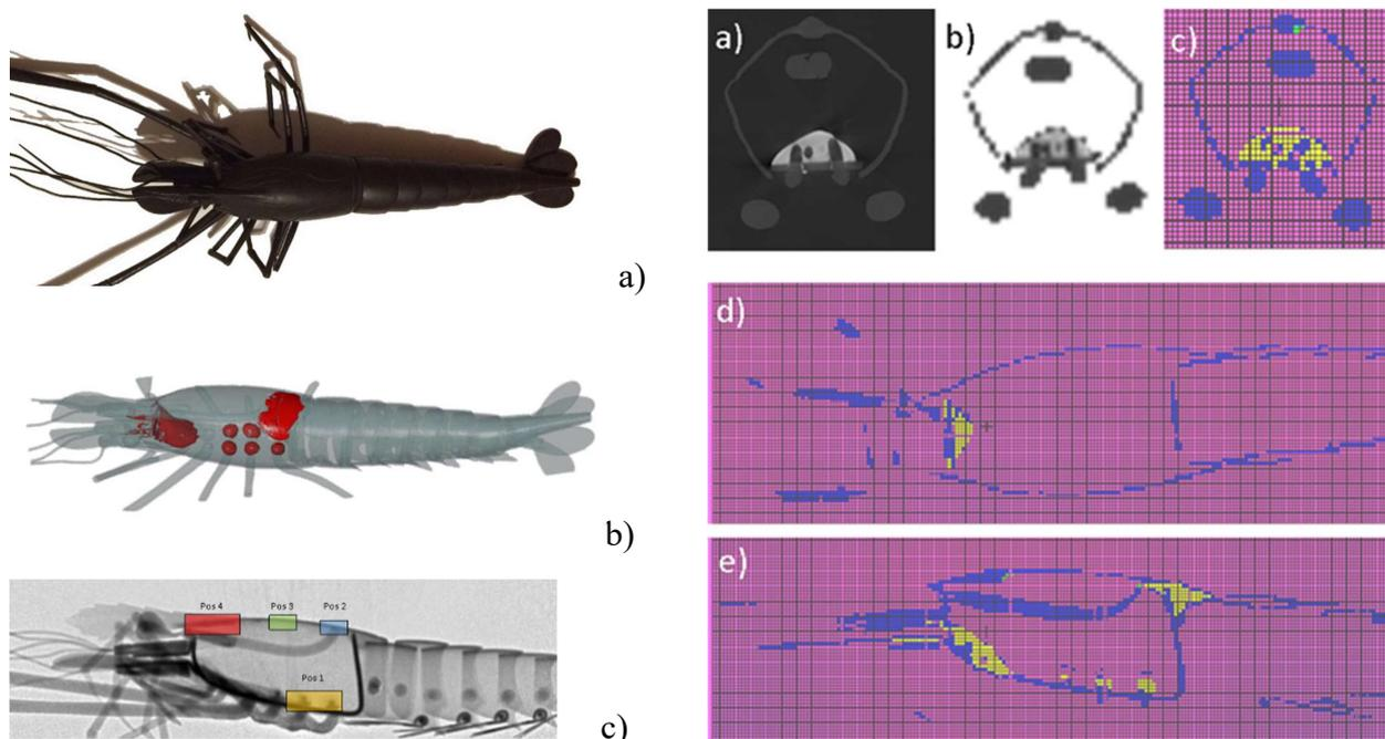
Figure 3. Left column: the photo, the segmented XCT, and the neutron-radiography-driven measurement positions of PGAA of the articulated lobster. Right column: The XCT slices (a) were segmented to discrete materials (b) and converted to MCNP geometry, shown at cutting planes (c-e). Materials are color-coded: air (purple), metal body (blue), solder1 (yellow), and solder2 (green).
