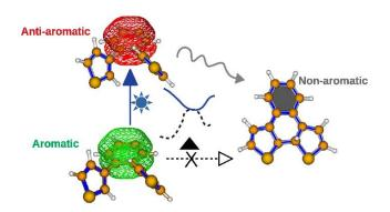
**Figure 5.** Photoinduced changes in aromaticity facilitate electrocyclization of dithienylbenzene switches.
