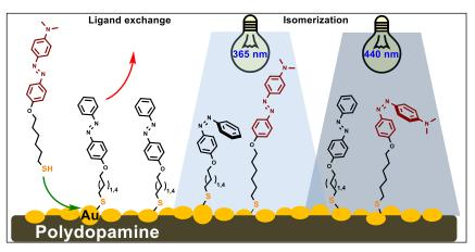
**Figure 2.** Photoswitchable macroscopic solid surfaces based on azobenzene-functionalized polydopamine/gold nanoparticle composite materials.
