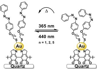
Figure 4. Light-induced and thermal isomerization of azobenzenes on immobilized gold nanoparticle aggregates.
