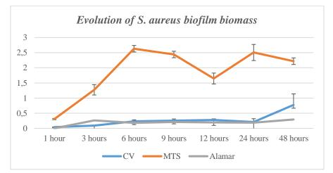
Evolution of untreated *S. aureus* biofilm biomass over time. The y-axis represents absorbance values which were measured spectrophotometrically, while the x-axis shows the different incubation periods when measurements were performed.
