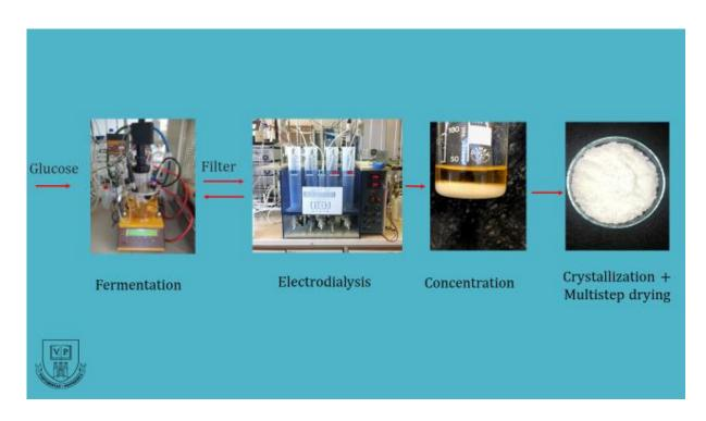
Figure 3: The complete process for itaconic acid production
