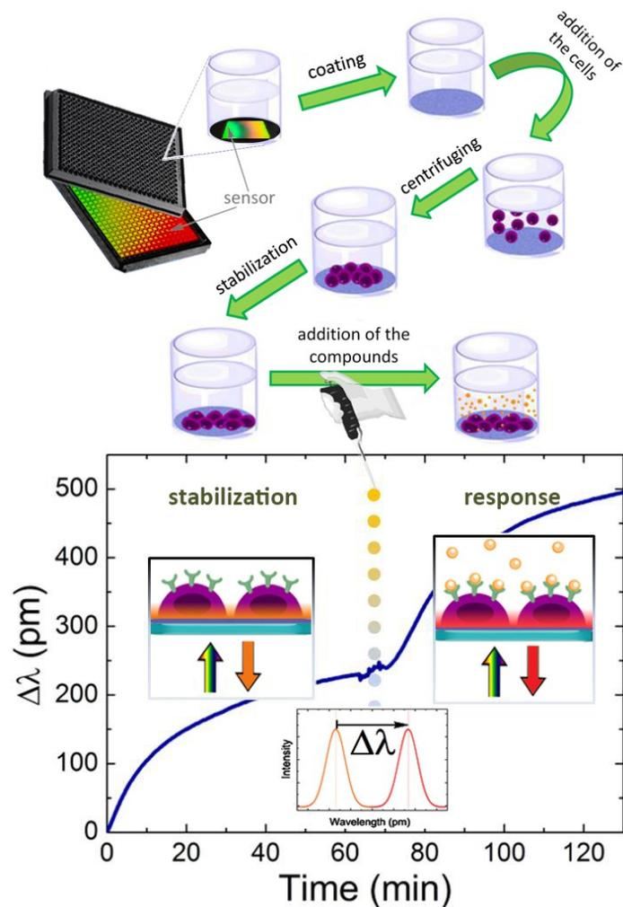
**Figure 1** Experimental setup to perform real-time measurement of dynamic mass redistribution (DMR) using B-cell lines (A); and schematic illustration of the principle of DMR detection (B)[1].
