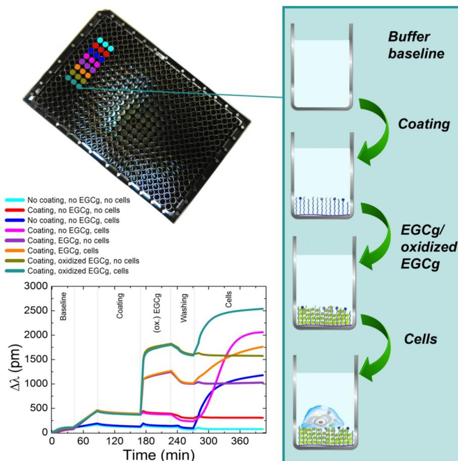
**Figure 1** In situ kinetic curves recorded by the Epic BT instrument. A 384-well plate used in the experiment is also shown, together with the manipulation steps in a typical well (right scheme). Typical experimental curves are plotted (bottom left corner) for PP:PPR coating, and 500  $\mu\text{g/ml}$  EGCg concentration. The detailed experimental conditions corresponding to the various kinetic curves are indicated above the graph.
