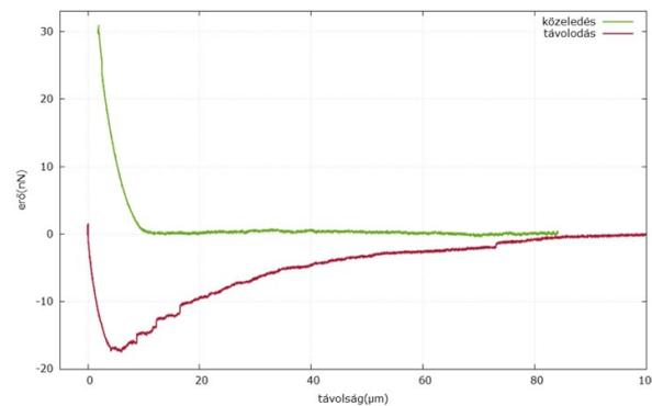
**Figure 2:** A typical single cancer cell adhesion curve from a FluidFM BOT measurement
