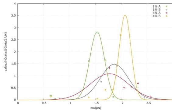
**Figure 1:** PDFs of adhesion forces from micropipette measurements on 4 different coatings
