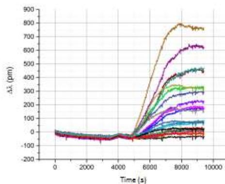
**Figure 2** Left: The biosensor signal distribution for a single HeLa cell. Right: The time series for the adhesion event for a single HeLa cell. The individual curves represents different  $21 \times 21 \mu\text{m}$  areas on the biosensor chip surface associated with the cell.
