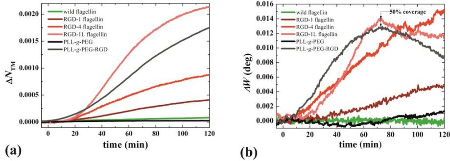
**Figure 2** OWLS signals recorded after living cells were seeded on the surfaces of the OWLS chips coated with the indicated layers. (a) The measured  $\Delta N_{TM}$  values correlating with the strength of cellular adhesion. (b) Temporal evolution of the width of the OWLS resonance peak ( $W$ ).
