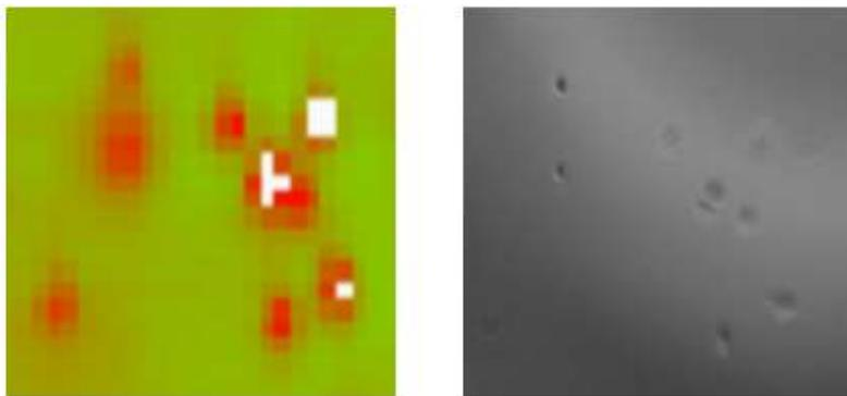
**Figure 1** The comparison between the biosensor signal distribution (left) and the microscope image (acquired with a phase contrast microscope, right) of the cells attached to the surface of the sensor.
