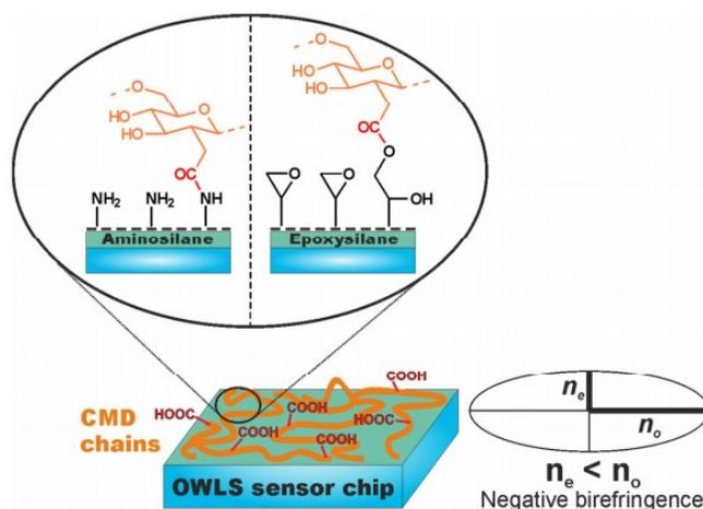
**Figure 1** Schematic illustrations of the CMD grafting chemistries and the supposed structure of the CMD chains on the OWLS sensor chip. The negative birefringence of the layer suggested lain down chains on the surface.
