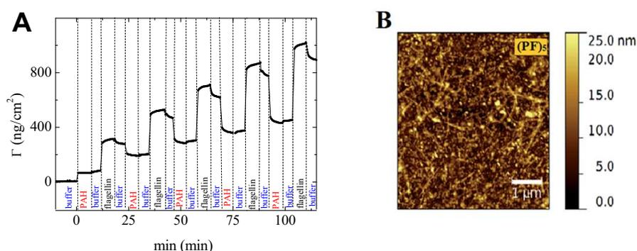
**Figure 1** shows A, Formation of 5 bilayer of flagellin and PAH polyelectrolyte monitored by OWLS. B, AFM picture of 5 bilayer of flagellin and PAH polyelectrolyte
