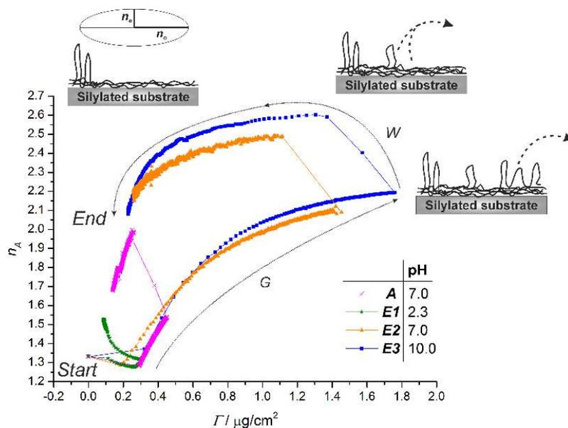
**Figure 2** In situ OWLS measurements on the covalent grafting experiments of the CMD ( $n_A$ : apparent refractive index of the CMD layer,  $\Gamma$ : areal mass density of the deposited CMD; A, E: surface with aminosilane or epoxysilane coating, respectively; G, W: grafting or washing sections of the experiment).
