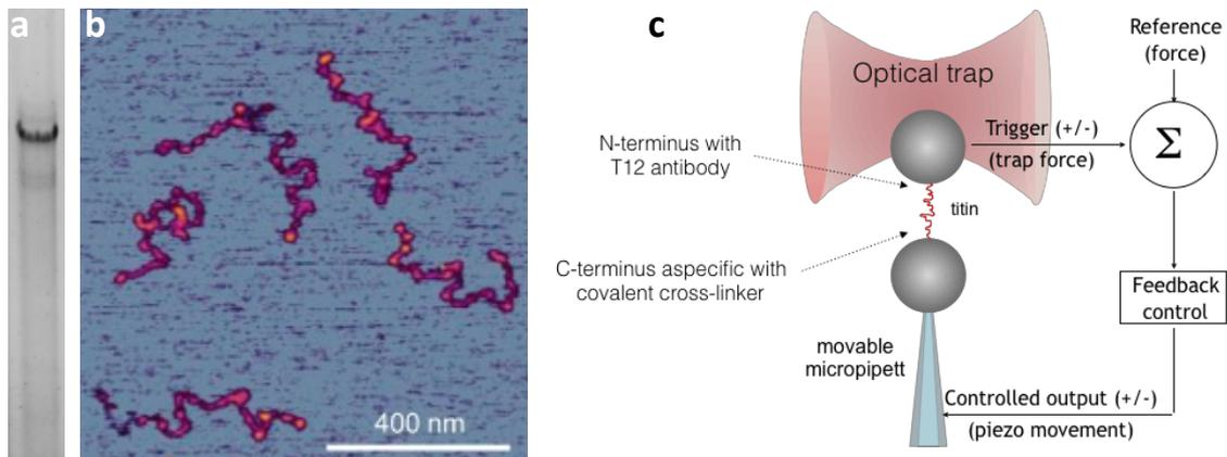
**Figure 2.** Isolation and manipulation individual titin molecules with force-clamp optical tweezers. **a.** 1% agarose gel profile of isolated titin. **b.** AFM image of isolated individual titin molecules. **c.** Experimental layout of titin manipulation and feedback control.
