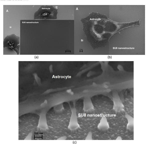
Figure 5.2. Primary mouse astrocytes avoid type A nanostructured SU-8 surfaces (a), while spread over type B nanostructured surfaces (b) and attach to spiky SU-8 nanopillars (c).
