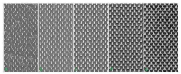
Figure 5.1. SU-8 nanostructures fabricated using different e-beam lithography parameters. The center-to-center distances are 500 nm.
