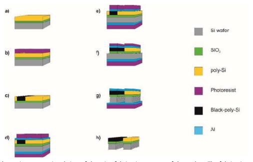
Fig. 3.1. Schematic cross sectional view of the microfabrication process of the probes. The fabrication steps are the following: a) thermal  $SiO_2$  growth (500 nm) and polycrystalline Si (1000 nm) deposition, b) photolithography: masking of the nanostructured parts, c) black Si formation by deep reactive ion etching d) deposition of an AI masking layer (300nm) and photoresist for device contour definition e) photolithography, AI etching, BI PolyBI and BI are the front- and backside.
