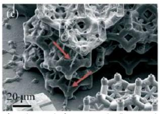
Fig.4.2. SEM micrographs of a tri-layer stack of structures with cells, neurites bridging layers and thereby creating 3D neuronal networks (denoted by red arrows).
