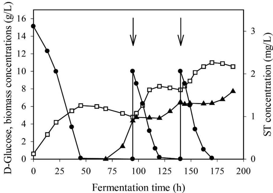
**Figure 3.** Time profiles of growth ( $\square$ ), residual D-glucose concentrations ( $\bullet$ ) as well as sterigmatocystin (ST) production ( $\blacktriangle$ ) in fed-batch fermentations of an *A. nidulans* wild-type strain in minimal media. Additional D-glucose (indicated by plain arrows) was added at 94 h and 140 h.
