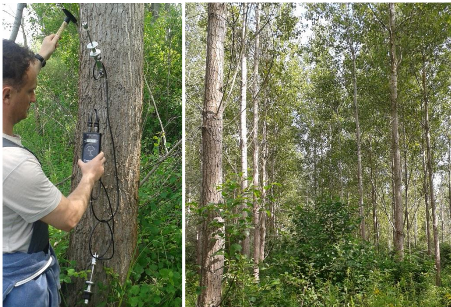
Figure 1 - On-site measuring with “Fakopp” TreeSonic device (left); Újrónafő 11G plantation (right)
