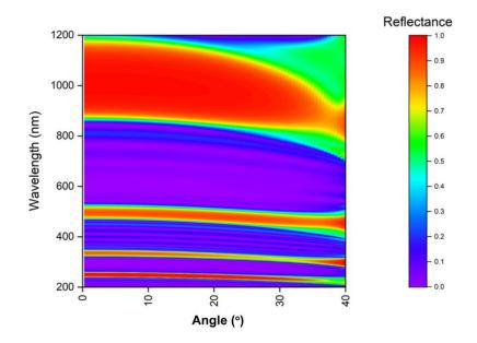
Intensity of the reflected light of different wavelengths in function of the incident/reflected angle. The structure consist of 7 pairs of 200 nm thin films (air and refractive index = 1.5). Angular resolution:  $0.5^{\circ}$ , wavelength resolution: 1 nm.
