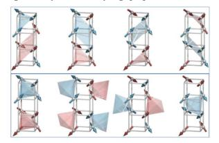
Magnetic ground state configurations simulated for Ru2MnZ (Z =Si,Sb) Heusler compounds with negative NN biquadratic coupling. The upper panel shows different variations of 3Q states, where the fully compensated (111) planes are indicated with red and blue colors. In the lower panel different variations of 4Q states can be seen, with fully compensated tetrahedra indicated by red and blue colors. [54]
