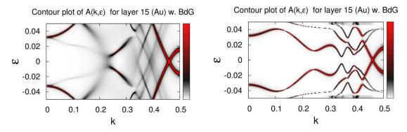
Contour plot of the BSF in the  $k_y=0$  direction corresponding the last layer of Au. The Au sample consisted 9 layers. The quasiparticle spectrum was calculated from the BdG equations.  $\Delta_{Nb}=0$  Ry is used on the left panel and  $\Delta_{Nb}=0.05$  Ry on the right panel. [6]
