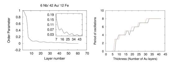
Left: Order parameter for the Nb/Au/Fe(001) system with 42 gold and 12 Fe overlayers. The inset shows the order parameter in the gold layers. The order shows an oscillating behavior with a period of 8 layers. **Right:** The oscillations' period of the order parameter as a function of the number of gold overlayers in case of 12 Fe (black line) and 24 Fe (red line) layers. [29]
