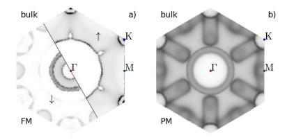
(a) Spin resolved spectral DOS of the ferromagnetic phase and (b) total spectral DOS of the paramagnetic phase of bulk Gadolinium at the Fermi energy as projected to the 2D Brillouin zone. Darker colors represent larger values of the spectral DOS. [2]
