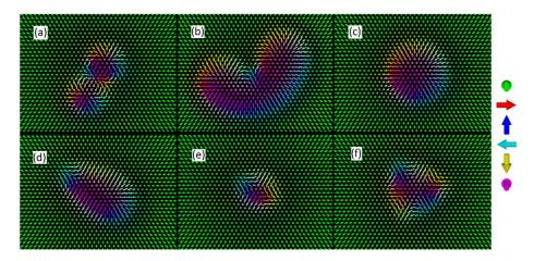
Metastable localized spin-configurations with different topological charges: (a) skyrmion with Q = -3, (b) skyrmion with Q = -2, (c) skyrmion with Q = -1, (d) chimera\_skyrmion with Q = 0, (e) antiskyrmion with Q = 1, and (f) antiskyrmion with Q = 2. The value of the external field is B = 2.35T in part (a) and B = 0.23T in parts (b)-(f); the ground state is field-polarized for B > 0.21T. The colors indicate the directions of the spin vectors, illustrated on the right edge of the figure. [22]
