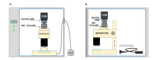
Fig 8. Laboratory built ultra low cost time lapse camera system
