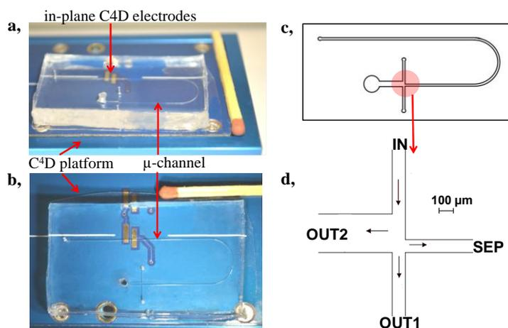
Fig. 2. A PDMS microchip with thin bottom layer ( $\sim 100 \mu\text{m}$ ) placed on the C4D platform to a position that the microfluidic channel crosses the two in-plane electrodes of the platform (top-side view (A) and top view (B)). The channel pattern includes a split-flow injection part for creating sample plug of subnanoliter volume in the separation channel (SEP) (C).
