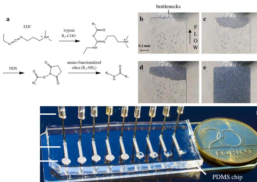
Fig. 4.(a) The covalent immobilization reactions with EDC/NHS between trypsin and amino-functionalized silica particles. (b–e) Optical micrographs of the packing formation process at the bottlenecks. The suspension of the silica particles in storage solution was pumped toward the bottlenecks. (f) Photograph of the microchip IMER with 9 simultaneous digestions. [8]
