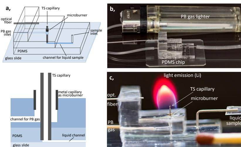
Fig. 5. Schematic construction of the miniaturized FAES system (left upper) and TS nebulizer/microburner (left lower) (a). Photographs of the miniaturized FAES system including microfluidic device and a propane/butane gas lighter (b) and the microfluidic device with flame colored by Li solution introduced via thermospray capillary (c) [10].
