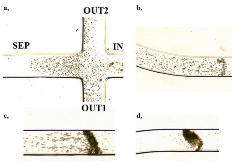
Fig. 6. Isotachophoretic separation/preconcentration of *Microcystis aeruginosa* bacterium cells in a microchip including a crossing of channels for injection of the cells (a.). Illustration of the zone sharpening effect due to ITP (b-d). These results are under publication.
