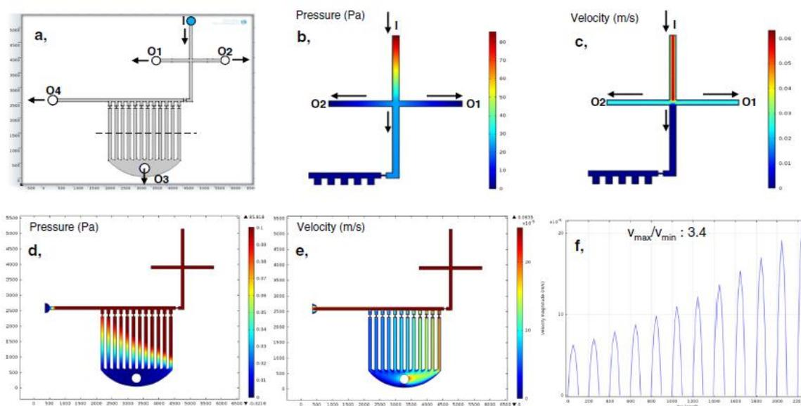
Fig. 1. COMSOL simulations of pressure distribution (b) and flow rates (c) in the sample introduction part (junction of fluid channels) and in the complete channel system (d, and e,) of the microchip. The flow rate applied at the inlet port I was 10  $\mu\text{L}/\text{min}$ , and the pressure at the outlet ports O1–O4 were set to 0 Pa [2].
