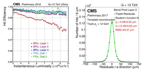
Figure 1: Left: Hit efficiency as a function of instantaneous luminosity in the pixel detector [6]. Right: Measurement of hit residuals in the new pixel detector [7].
