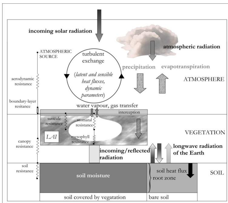
Fig. 8. Flow chart of the deposition model
