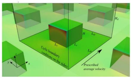
Figure 2. Schematic of the geometrical setup for the series of numerical simulations.
