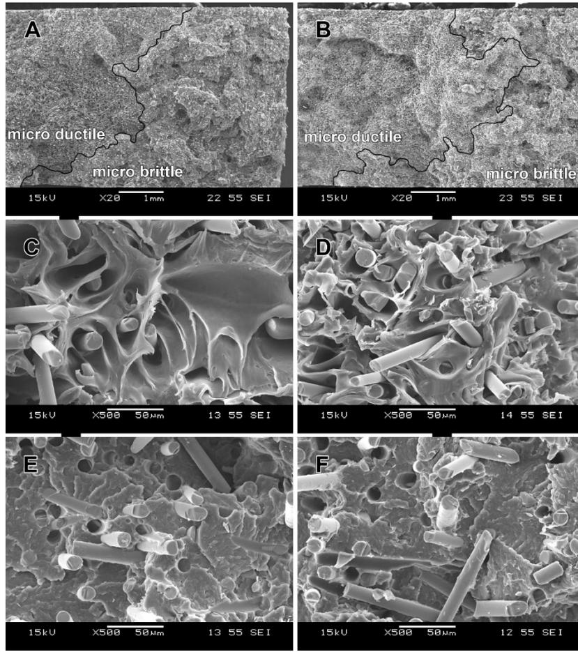
Fig. 6. Typical fracture surface of the PA6 / 30 BF composite (A, C, E) and hybrid composite with 0.25 wt% GnP content (B, D, F).
