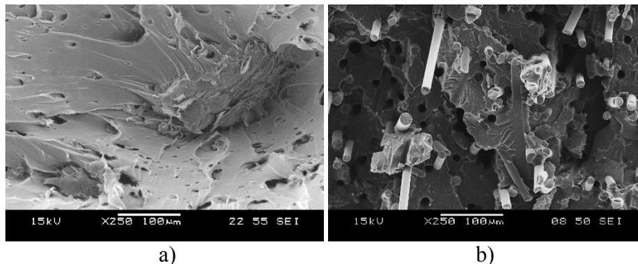
Fig. 3. Fracture surfaces of tensile tested composites:
