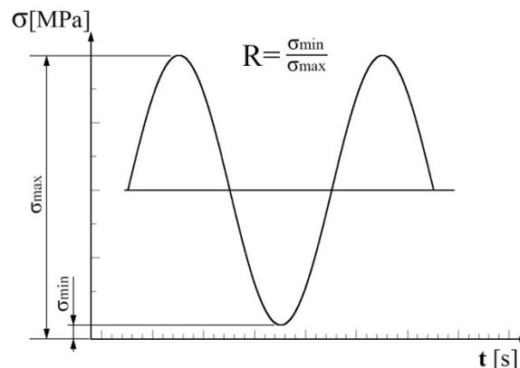
Fig. 1. Tension-tension fatigue test load as a function of time
