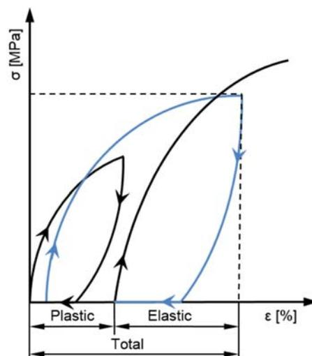
Fig. 2. Strain-stress curves for cyclic loading, at increasing load levels (the blue colored curve signs a complete cycle)
