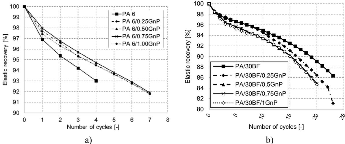
Fig. 5. The elastic recovery as a function of cycle numbers:
