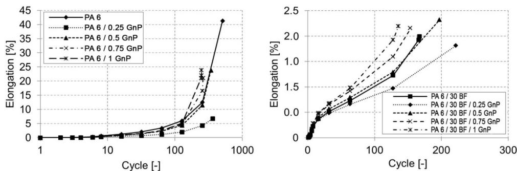
Fig. 4. Elongation as a function of cycle numbers in case of fatigue tests: a) PA6 / GnP nanocomposites; b) PA 6 / 30 BF / GnP hybridcomposites
