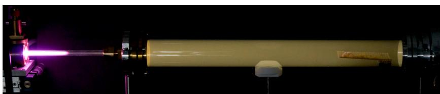
Figure 1: The post-discharge system with the surface-wave microwave discharge operating in  $N_2$ -20% $O_2$  mixture during seed treatments.
