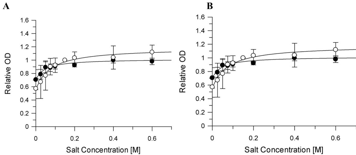
**Fig 1.** Effect of salt concentration on collagen coating.
