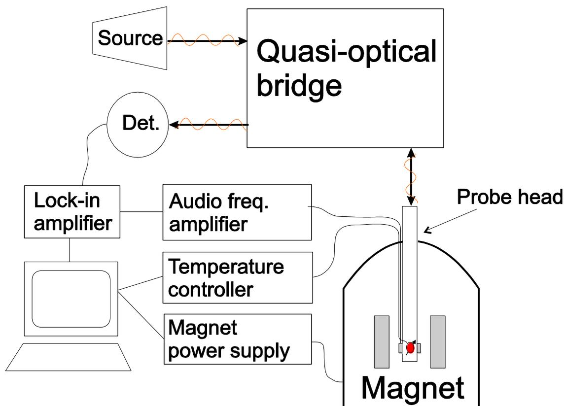
Figure 2. Block diagram of the spectrometer. The quasi-optical bridge transmits the microwaves from the source to the probe head. It filters the signal from the reflected radiation and directs it to the detector. The audio frequency amplifier drives a small coil in the probe head that modulates the magnetic field and the signal of the detector is processed by a lock-in amplifier. The measurement is controlled by a PC.
