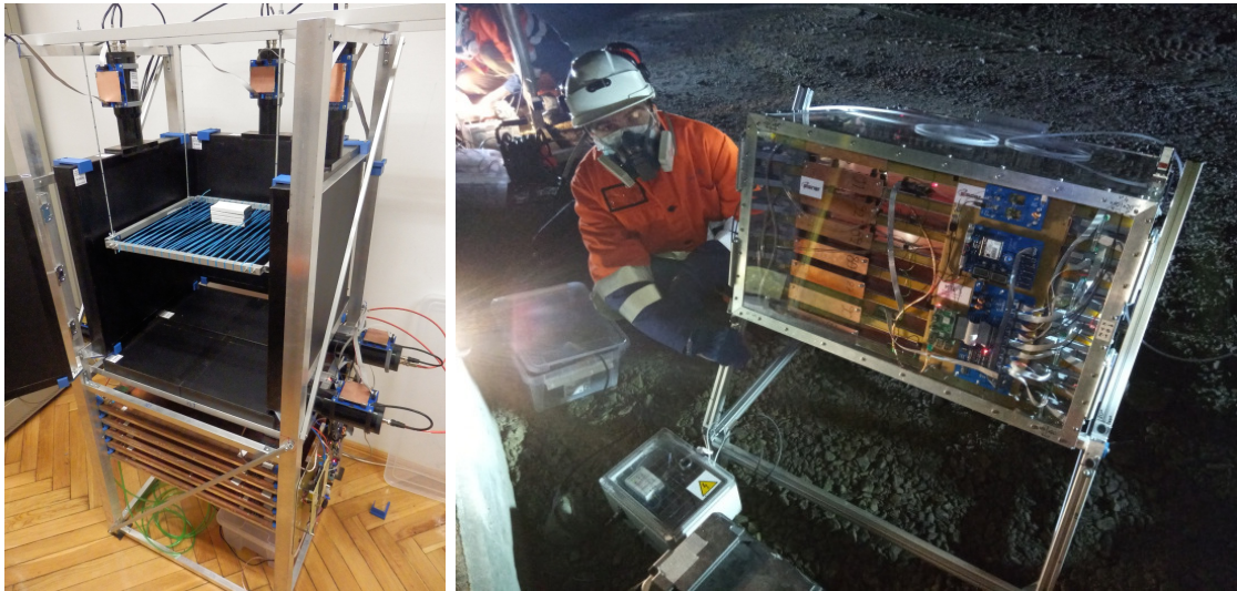
Figure 2: Left: Photo of the COMIS experiment in Budapest, secondaries are detected in the surrounding plastic scintillators, while the underlying trackers give position information. The combined DAQ system makes it compact and simple.
