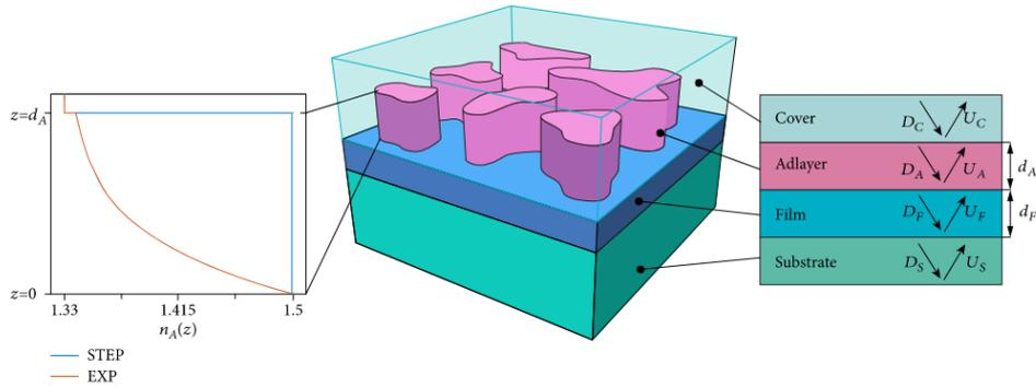
**Figure 13.** The structure of the modeled OWLS waveguide chips with inhomogeneous adlayer. The modeled multilayered assembly consists of 4 layers: substrate, waveguide film, adlayer, and cover.
