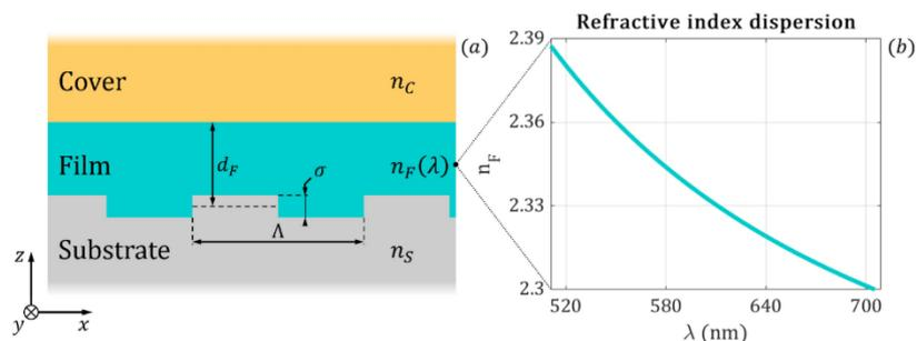
**Figure 14.** (a) The cross-section of the modeled corrugated waveguide. The electromagnetic simulations apply Floquet boundary conditions along the  $x$ - and  $y$ -axis and open boundaries with Floquet ports in the vertical  $z$  direction. (b) The frequency dependence of the Nb<sub>2</sub>O<sub>5</sub> film refractive index.
