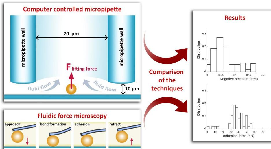
**Figure 2.** Schematic illustration of the methods. Adhesion force measurements on microbeads were performed by using computer controlled micropipette (CCMP) and Fluidic force microscopy. The received results of the two techniques has been compared.
