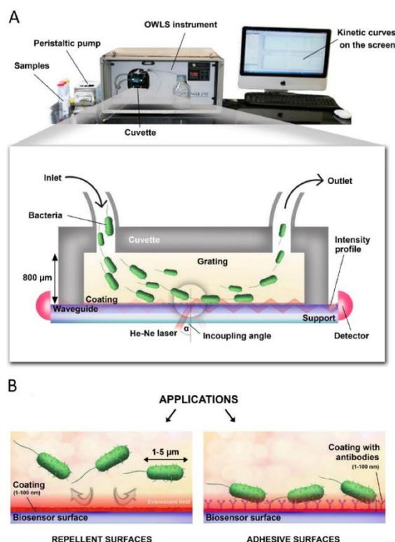
**Figure 6.** (A) Cross-sectional view of the OWLS cuvette and the basics of optical detection. Laser light is coupled into an optical waveguide layer by a surface grating where it propagates by total internal reflection to a photodetector placed at the end of the waveguide. Adsorbing bacteria shift the resonant angle ( $\alpha$ ). (B) OWLS is an ideal tool for testing and developing both bacteria repellent and bacteria adhesive surfaces.
