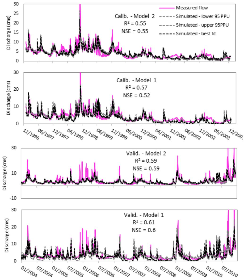
**Figure 7.** Calibration and validation results for the Zalaapáti gauge for the two model variants.
