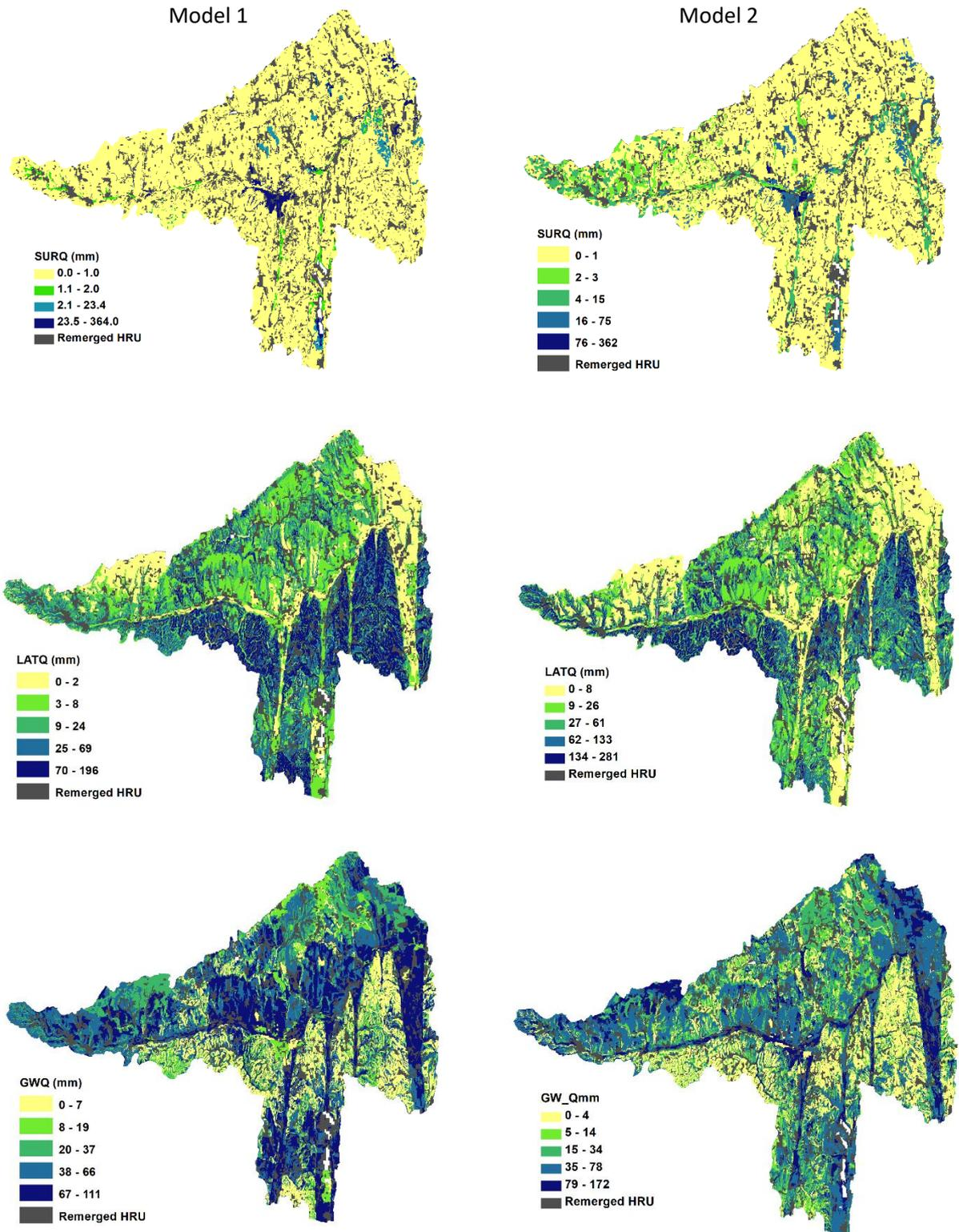
**Figure 8.** – Spatial distribution of runoff components as a result of two model variants (SURQ – surface runoff, LATQ – lateral flow or interflow, GWQ - groundwater flow).
