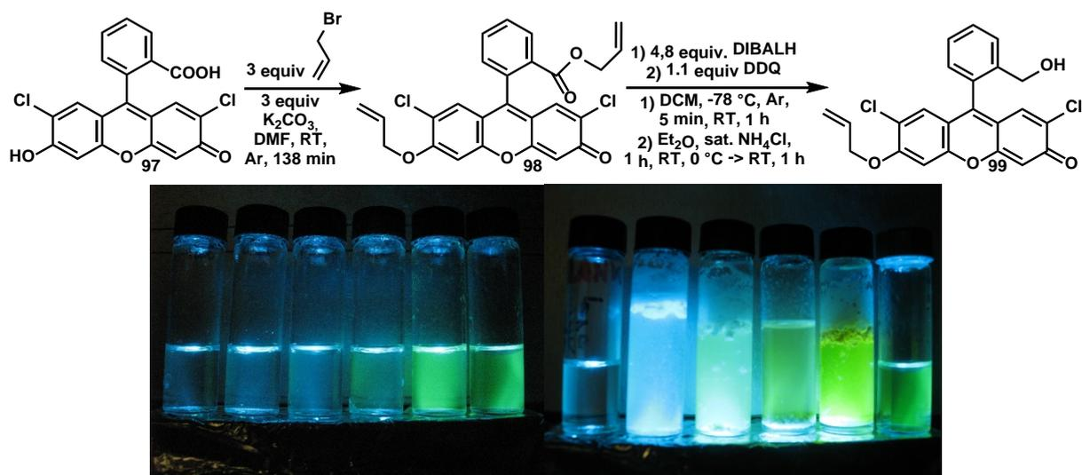
**Figure 1a:** Analysis of palladium stock solutions by fluorogenic Tsuji-Trost reaction, Pd concentration of vials, from left to right: 1  $\mu\text{g}/\text{kg}$ , 10  $\mu\text{g}/\text{kg}$ , 100  $\mu\text{g}/\text{kg}$ , 1 mg/kg, 10 mg/kg, 100 mg/kg
