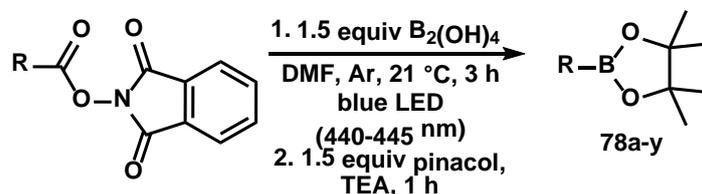
**Scheme 4.** Photocatalytic transformation of active esters to boronates under visible light irradiation
