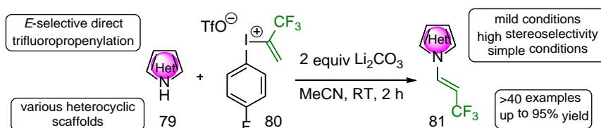
**Scheme 15.** Synthesis of trifluoropropenylated heterocycles
