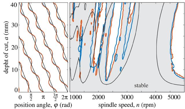
Fig. 2. Montage of the results achieved in NKFI PD 124361 project related to milling processes.
