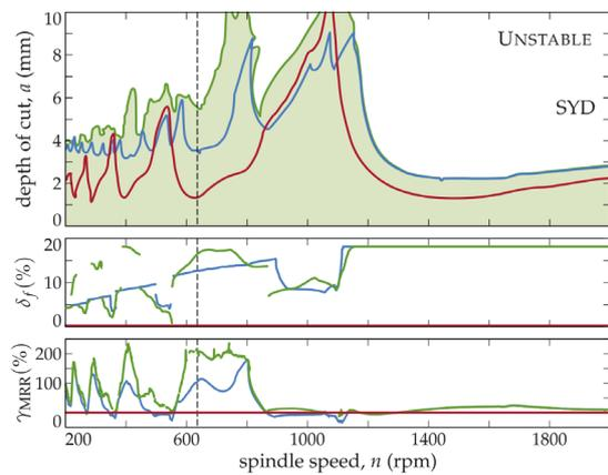
e) new harmonically varying milling tool model [10]
