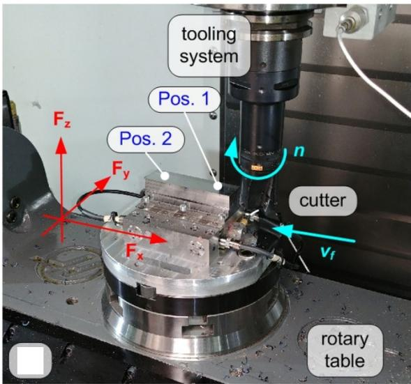
b) model of general active milling process [18, 17]
