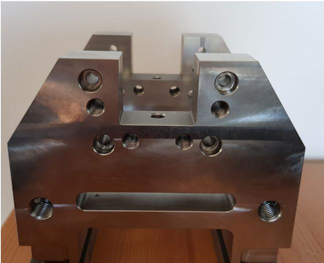
b) retrofitted rolling machine roller guide system
