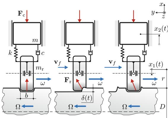
b) axles rolling model shows stable and unstable rolling [19]
