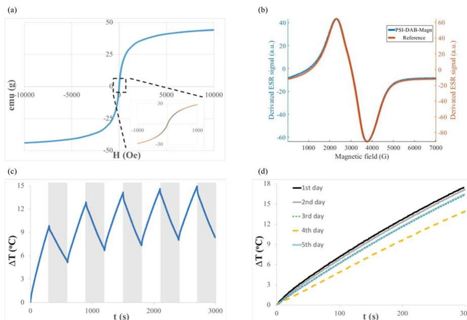
**Figure 5. a) SQUID study of the crosslinked magnetite loaded fibrous sample. (b) The ESR signal of magnetite matches the reference signal. (c) The change in temperature of the sample during five 5 minutes heating-5 minutes cooling hyperthermic measurement cycle. (d) The change in temperature of the sample during the 5-day repeated hyperthermic measurement.**
