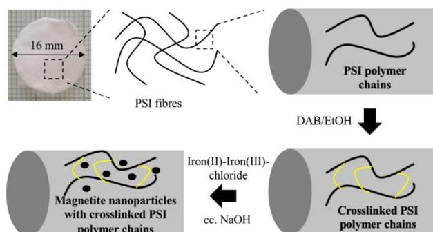
**Figure 4. Schematic representation of the chemical treatment of the fibrous scaffold-magnetite synthesis.**
