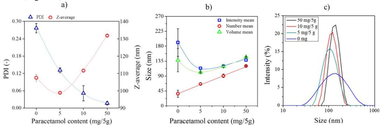
**Figure 2. Effect of paracetamol on properties of silver nanoparticles a) polydispersity index (PDI) and z-average b) particle size and c) intensity-based size distribution.**
