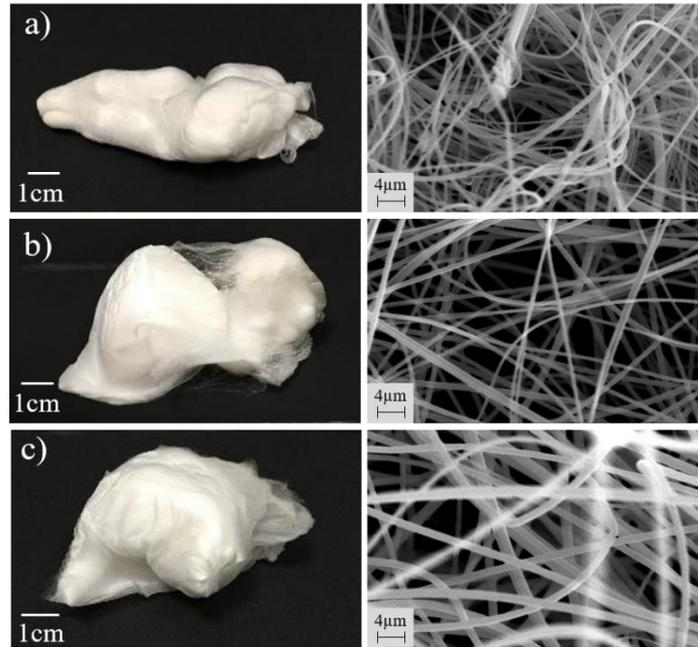
**Figure 9. Macroscopic picture of the 3D effect of different salts used and their SEM pictures on the right a) LiCl 1 w/w% b) MgCl<sub>2</sub> 1 w/w% c) CaCl<sub>2</sub> 2 w/w%. The scale on the SEM images correspond to 2μm.**
