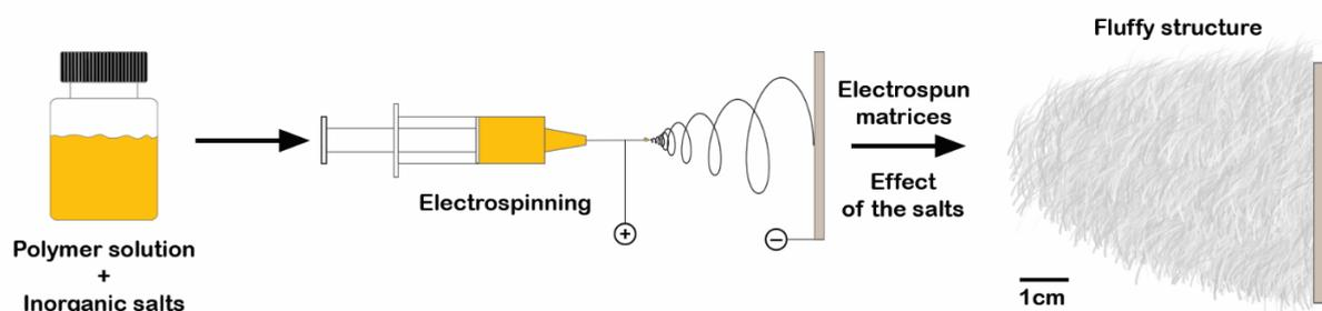
Figure 7. Schematic representation of the 3D scaffold preparation using electrospinning technique.
