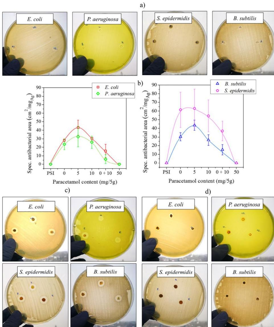
Figure 3. a) Kirby-Bauer or Disc diffusion method using PSI membranes b) Specific antibacterial area of silver nanoparticles within electrospun meshes and diffusion zone of c) the most effective sample: 5 mg/5 g APAP meshes d) the least effective sample: 50 mg/5 g APAP meshes with all tested bacteria strains.
