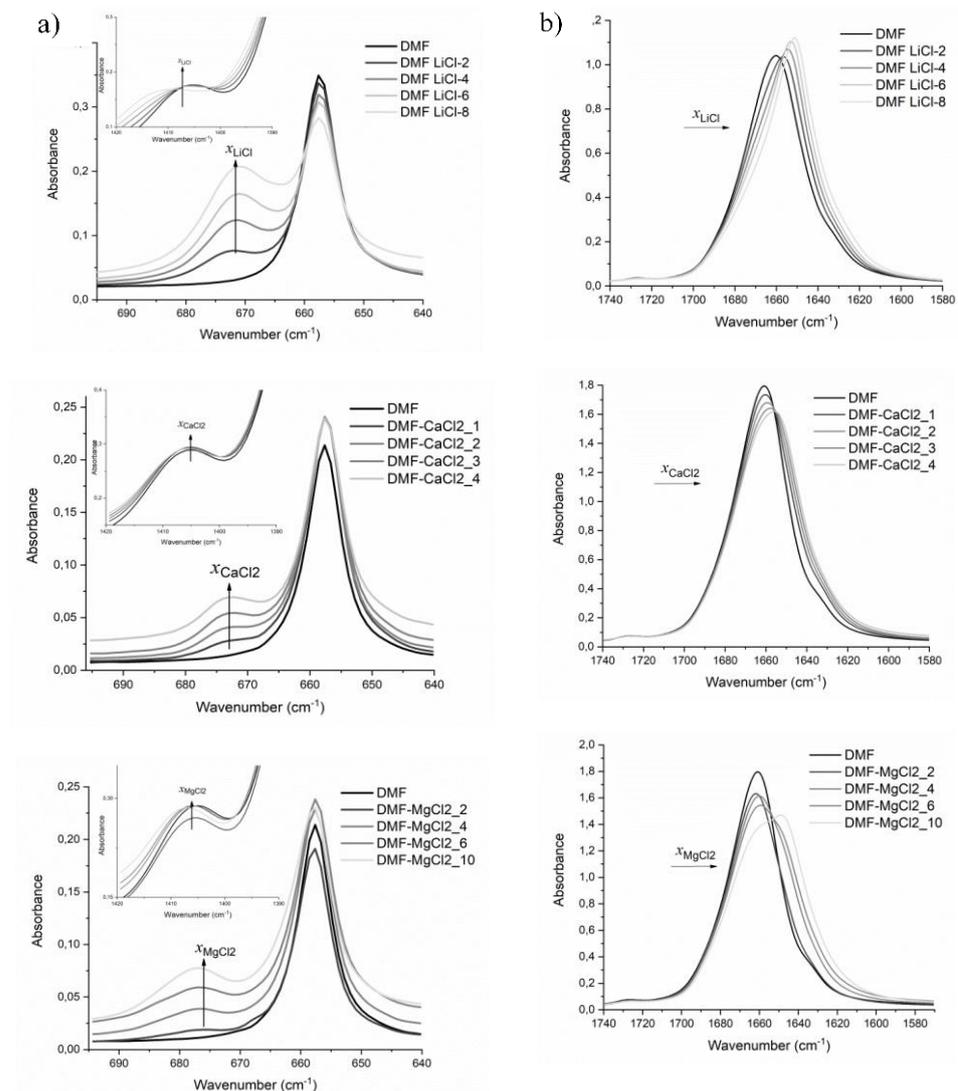
**Figure 8** IR spectra of the NCH=O a) and the C=O b) vibration modes in mixtures of LiCl (2, 4, 6 and 8 w/w%) CaCl<sub>2</sub> (1, 2, 3 and 4 w/w%) and MgCl<sub>2</sub> (2, 4, 6 and 10 w/w%) with DMF.
