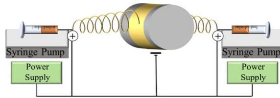
**Figure 1. A theoretical NP coverage with polymer and APAP (a) and the fiber formation (b). In the lower schematic draw represent a two-needle electrospinning setup for the fabrication of nanofibrous meshes.**
