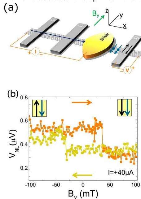
Figure 4. Spin injection using BiTeBr into graphene. a) Device sketch and a non-local measurement in b).
