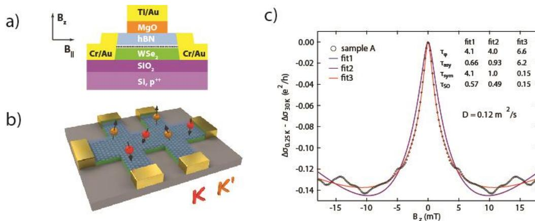
Figure 5. Induced spin orbit in graphene/WSe<sub>2</sub> heterostructures. a) Sketch of the device under study. b) Artistic view of the Hall bar with the effect of valley Zeemann term on the spins. c) WAL measurement with the fit parameters shown in the legend.
