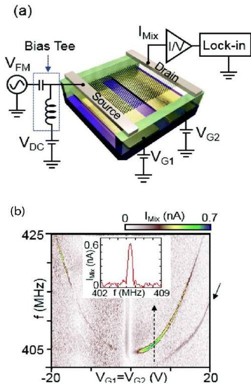
Figure 2: a) Schematics of suspended graphene resonator with the measurements circuit. b) Measurement of a lower frequency resonator. The plot shows the mixing current as a function of frequency and gate voltage with the large currents represent the resonance condition.
