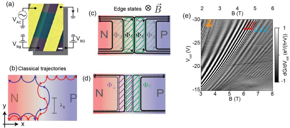
Figure 1. Magneto oscillations in high-mobility graphene pn junctions. a) False coloured SEM image of graphene pn junction. b) Sketch of classical snake states. c)-d) Mach Zehnder interferometers defined by edge states. e) Measurements on a p-n junction showing a wealth of magneto-oscillation effects.
