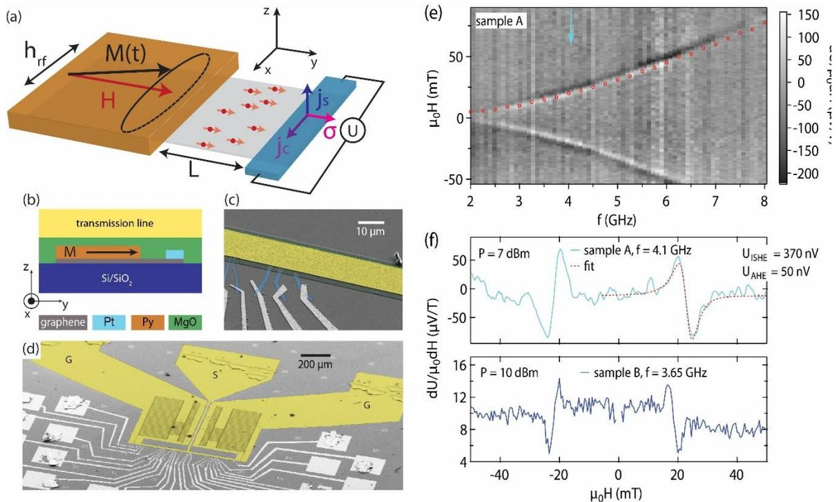
Figure 3. Spin pumping into graphene. a) sketch of the device with the precessing ferromagnet on the left, and the Pt electrode with the inverse spin Hall effect on the right. b) side view of the device c-d) False coloured SEM images of the device. e) Spin hall voltage as a function of magnetic field and excitation energy. f) Cut around 4GHz, and the result for another device.
