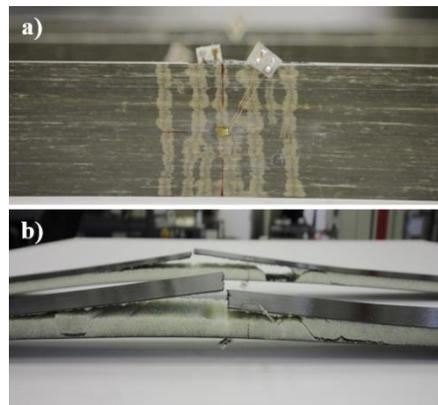
Figure 5. a) activated overload sensor, b) post mortem image of the sandwich beam specimens
