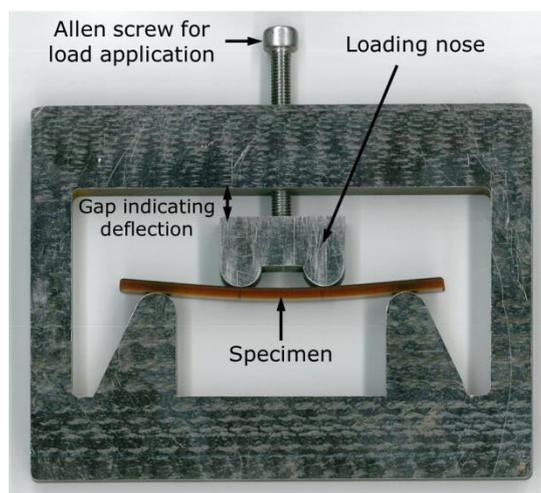
Figure 2. Four point bending frame for microscopy under deformation [10]
