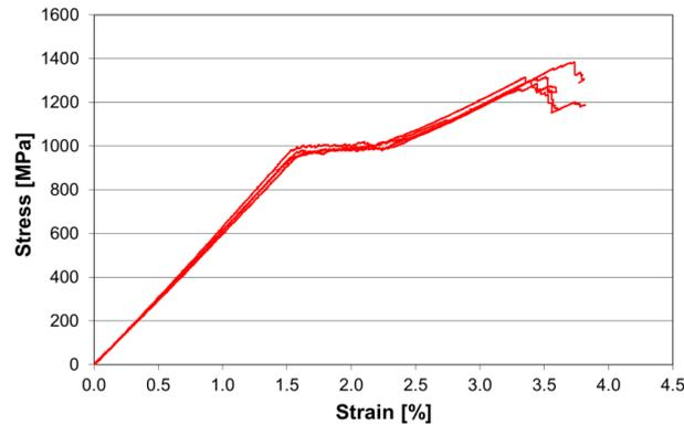
Figure 1. Pseudo-ductile tensile stress-strain response of continuous thin-ply glass/carbon fibre hybrid composite specimens [5]
