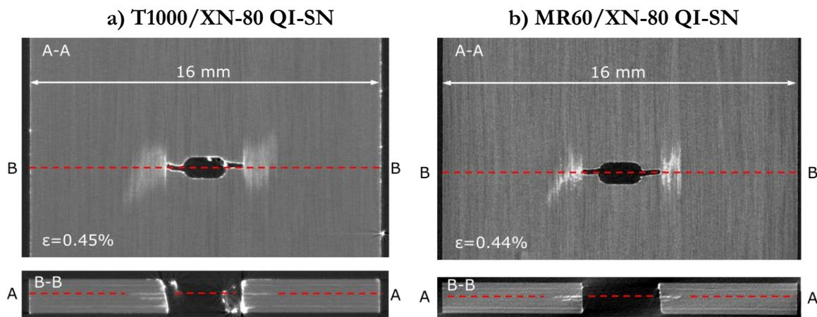
Figure 1. Full width X-ray CT scans of different type notched specimens after tests interrupted before any stress-drop at the overall strains indicated on the scans. Top view scans show the damage in one of the  $0^\circ$  sublaminates. [8]
