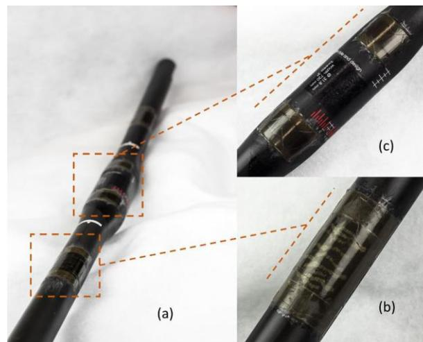
Figure 4. Bike handlebar fitted with hybrid composite overload sensors: (a) MTB Racing flat handlebar, retrofitted with (b) long single layer (c) short single layer sensors [12]
