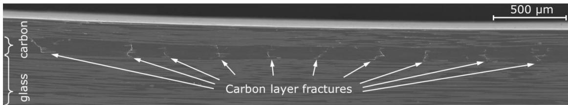
Figure 3. Carbon layer fractures on an edge view scanning electron micrograph [10]
