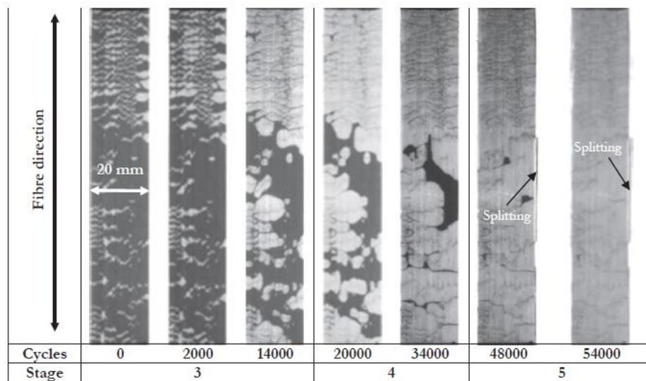
Fig. 6. Typical fatigue damage development of an overloaded UD thin-ply hybrid composite cycled at 70% of the damage initiation stress [13]
