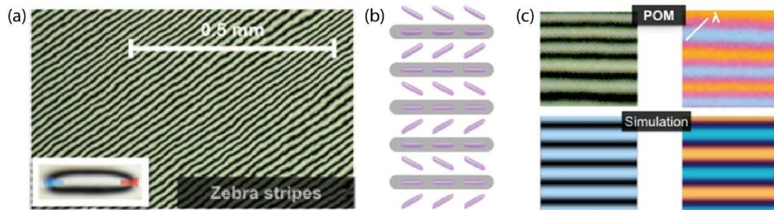
Figure 2: (a) Large scale topological pattern observed in polarized optical microscopy (POM); inset: the two ends of an elongated stripe are of one-half topological strength defects with opposite topological charge. (b) A schematic of the director field of the stripes. (c) A detailed POM view and a simulated image of the Zebra stripes with crossed polarizers, and with a  $\lambda$ -plate inserted. The simulation is made by the Jones matrix method.
