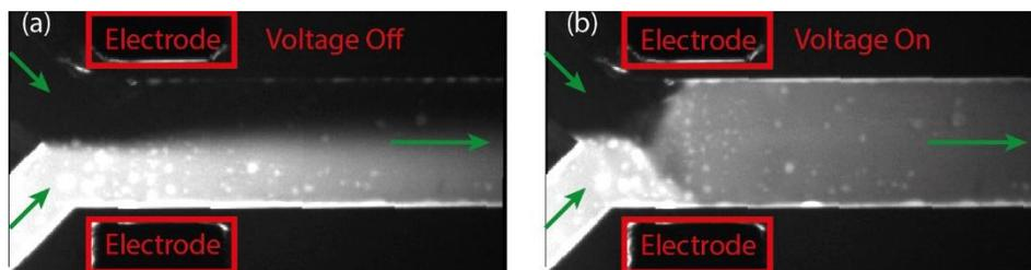
*Figure 1: Observation the mixing of two identical liquid crystals in a microfluidic Y-junction by fluorescent microscopy. The lower branch is doped with a fluorescent dye. (a) Mixing by diffusion. (b) Mixing by electroconvection. The width and depth of the merged channel was 100  $\mu\text{m}$  and 10  $\mu\text{m}$ , respectively.*
