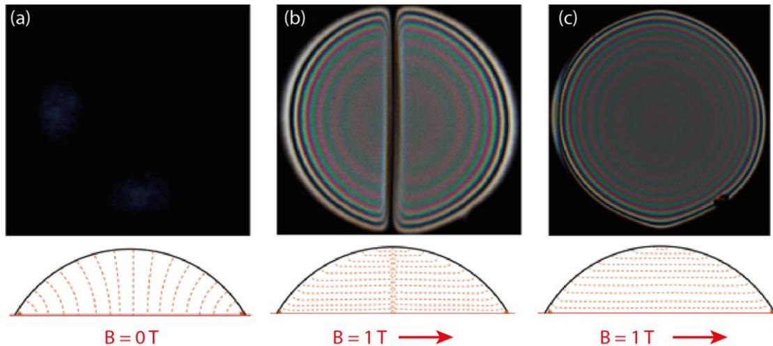
Figure 3: Top view of textures between crossed polarizers at  $\pm 45^\circ$  with respect to the magnetic field (horizontal) of a  $490 \mu\text{m}$  diameter liquid crystal drop illuminated by white light, and the corresponding director structure in side view, with (a) no magnetic field, (b)  $B = 1 \text{ T}$  with an inversion wall in the middle, and (c)  $B = 1 \text{ T}$  with the inversion wall moved to the left side.
