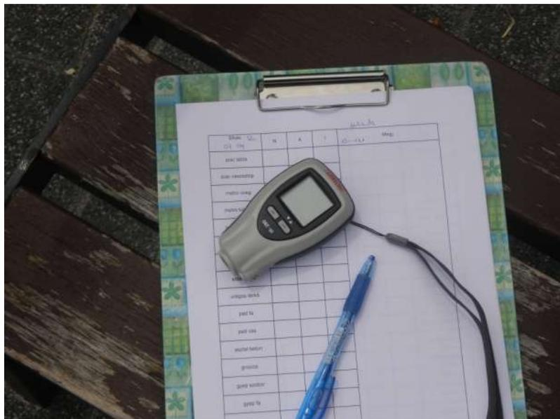
Fig. 10: Voltcraft IR-280 infrared thermometer used for measuring surface temperature.
