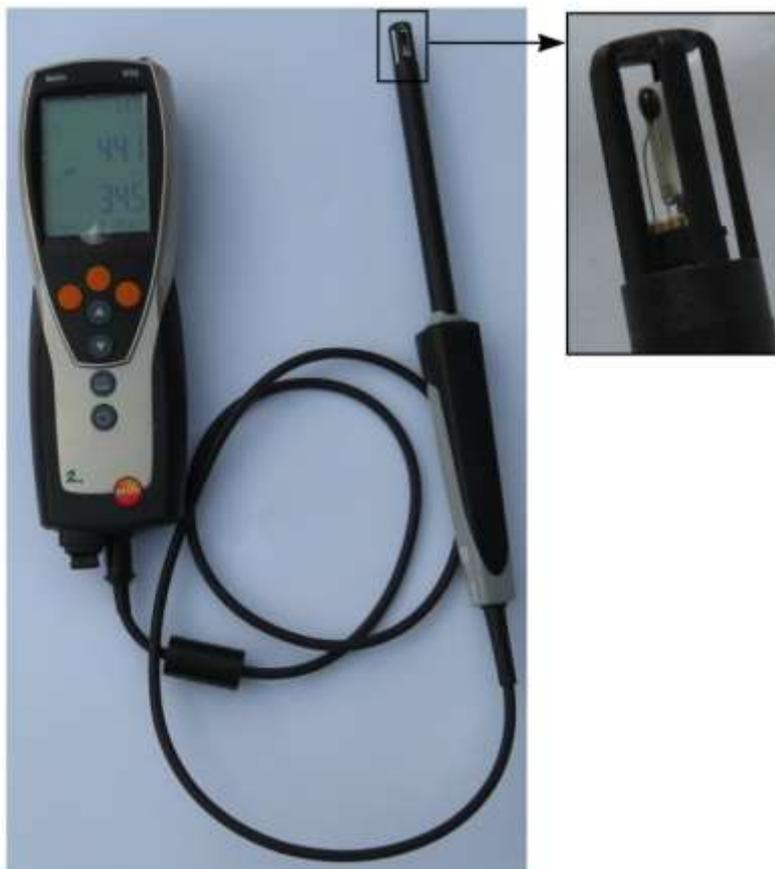
Fig. 2: The complex measuring instrument Testo-623 with data logger
