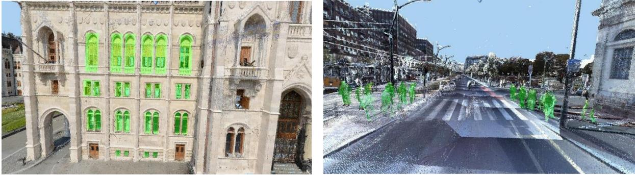
**Fig 1.** Demonstration of the large point cloud visualization and manipulation tool developed in the project. Left: annotated windows in the 1.5 billion sized point cloud of the Hungarian Parliament. Right: annotated pedestrians by Deák Square Budapest. MLS test data has been provided by Buda pest Közút Zrt.
