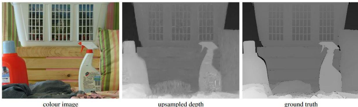
**Fig 3.** Result of an upsampled depth map (center), to a high resolution optical image (left), with available ground truth depth information (right)
