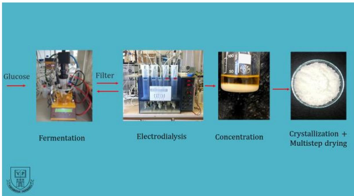
Figure 3: The complete process for itaconic acid production
