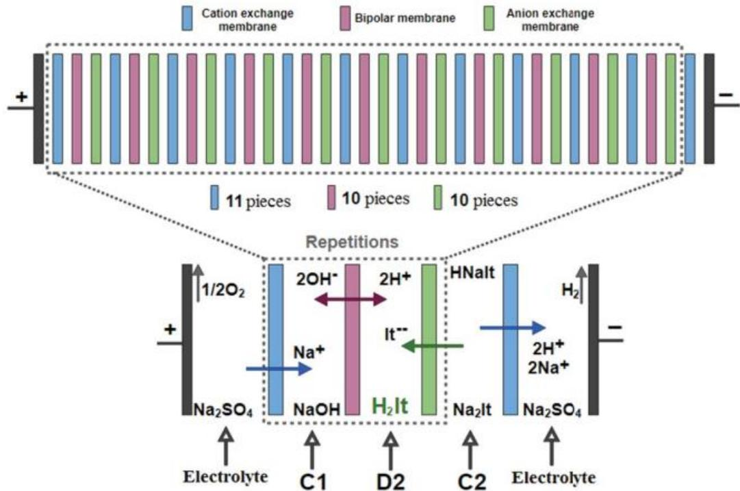
Figure 2: The scheme of the bipolar electro dialysis system
