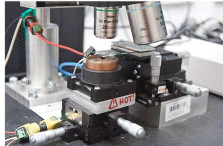
**Fig. 2 Stacking setup** (Left) Optical microscope which allows the visual control on the stacking process. (Right) Stage with micromanipulators, where different 2D layers from pdms/ppc mask can be positioned and released by local heating.
