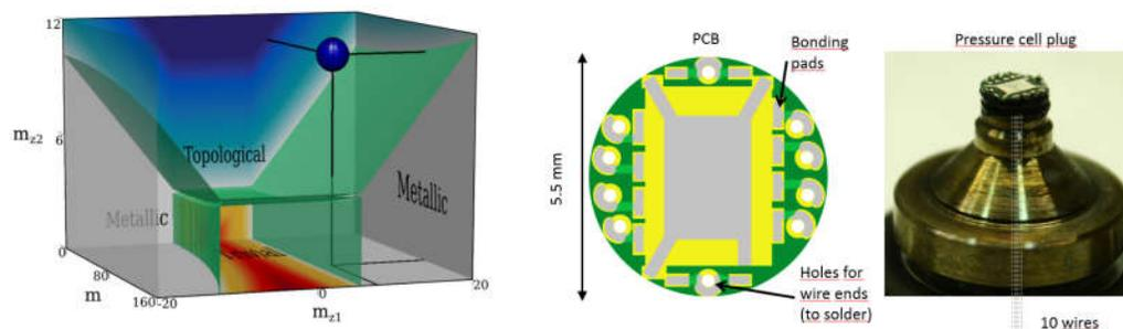
**Fig. 6 Heterostructures under strain** (Left) Topological phase diagram of graphene/BiTeBr structure. The electron structure of the system shows a reach phase diagram as in-plane uniaxial strain or out-of plan stress is applied. [6] (Right) Parts of the developed pressure cell, which allows to study nanocircuits under pressure. Small PCBoard is integrated on the plug of the cell, which hosts the silicon chips. [d7]
