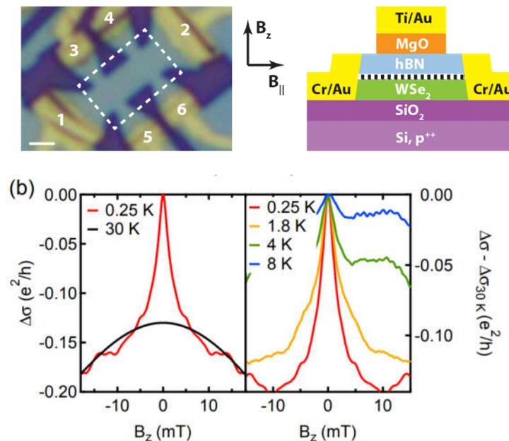
**Fig. 5 Weak anti-localization of graphene/WSe** (Up) Device geometry: graphene is encapsulated between WSe<sub>2</sub> and hBN, which results high mobility. (Down) Resistance as a function of external perpendicular magnetic field averaged in a gate voltage window. At low temperatures the resistance shows a peak at  $B_z=0$ , which is resulted by weak antilocalization effect. It is a signature of proximity spin-orbit interaction.
