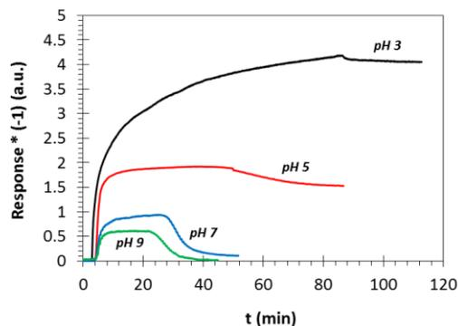
**Fig. 10.** PRiFS sensorgrams in the case of pH=9,7,5,3 AuNP(-) gold sol on the surface of PEI functionalized  $\text{SiO}_2$  nanoparticles (prepared by Langmuir-Blodgett method).
