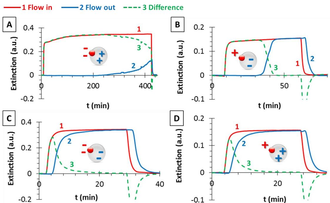
**Fig. 8.** Investigation the role of the surface charge: (A) negatively charged Au nanoparticles (AuNPs) on the surface of functionalized, positively charged glass beads (GB); (B) interaction of AuNP+ and GB-; (C) interaction of AuNP- and GB-; (D) interaction of AuNP+ and GB+.
