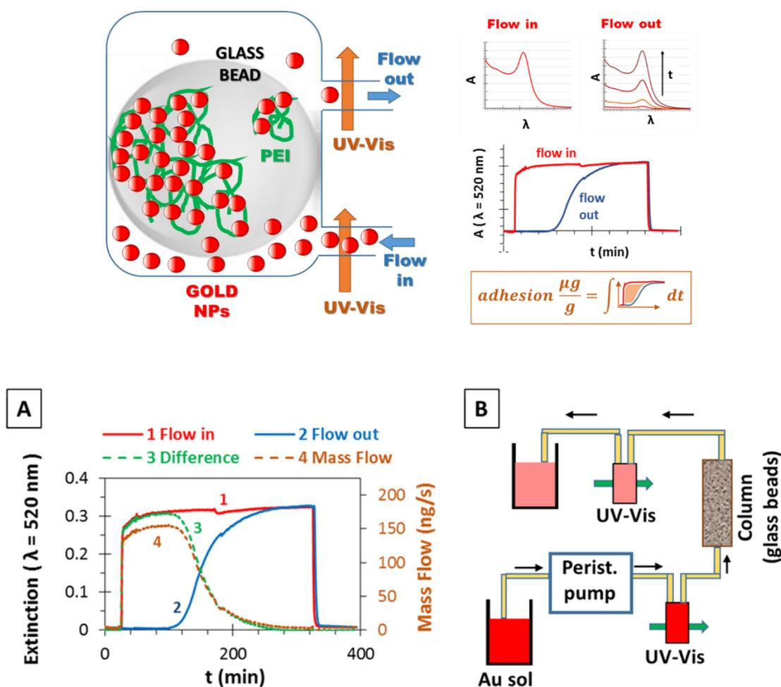
**Fig. 7.** The graphical abstract of the article (upper); the schematic view of the measurement principle (A) and the setup (B): the determination of the adhered gold nanoparticle amount on the surface of the original and functionalized glass beads is based on the differential measurement of the flow-in and the flow-out extinction/concentration values.
