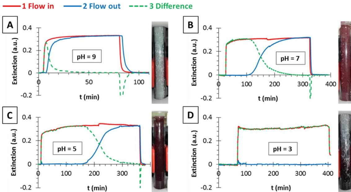
**Fig. 9.** Investigation the role of the pH of the (AuNP-) gold sol: (A) pH=9; (B) pH=7; (C) pH=5; (D) pH=3. The decreasing pH value causes strongly increasing negative surface charge, therefore strongly increasing adhered amount of AuNPs.
