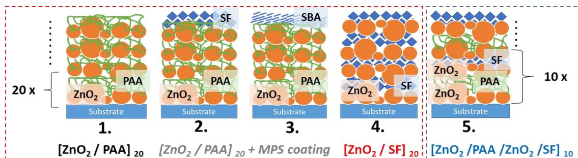
**Fig. 1.** The schematic view of the prepared and applied hybrid thin films. (*Fig. 2. in publication*)
