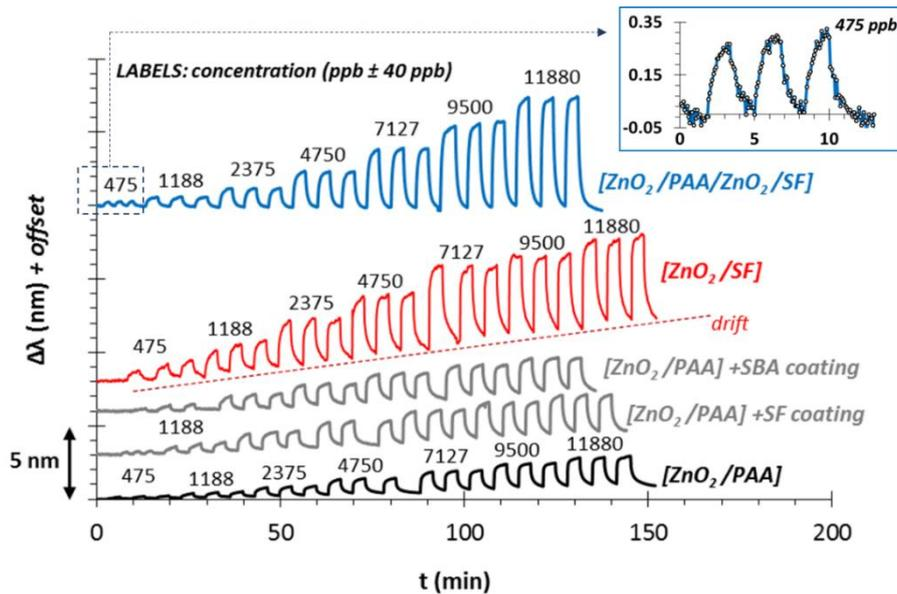
**Fig. 2.** Ethanol sensing tests:  $\Delta\lambda$  vs.  $t$  curves for the tested thin films (labels: structure of the thin film and the ethanol concentration steps); inset: response of  $[\text{ZnO}_2/\text{PAA}/\text{ZnO}_2/\text{SF}]_{10}$  mixed structure for  $c=475$  ppb EtOH (Fig. 6.a in publication).
