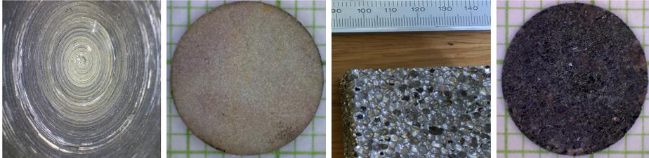
FIGURE 1. The heterogeneous structure of the measured materials. From left to right: capacitor, limestone from Villány, metal foam, leucocrata rock with slires.
