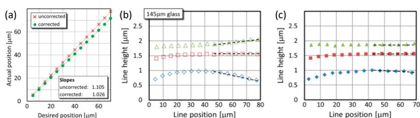
Figure 1: Improvement of focal position shift (a) and correction of focal shape distortion during polymerization through thick photoresist layer (b, c).
