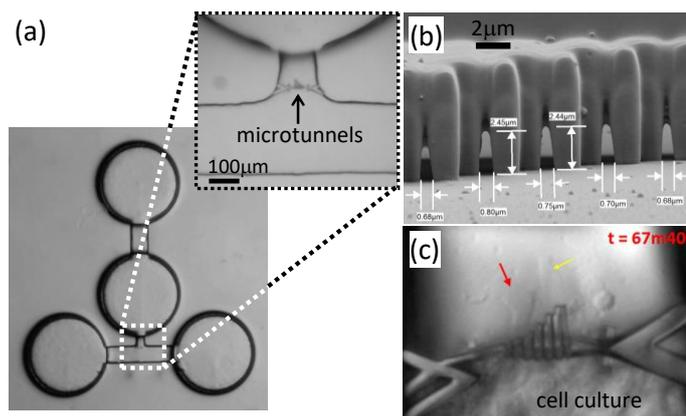
Figure 3: LOC chip to study cell migration (a); insert: localization of the microchannels in between the two functional regions. SEM image of  $\sim 0.75\mu\text{m}$  wide channels (b). Snapshot of a cell migration experiment; the two arrows are pointing to two cells already on the other side (c).
