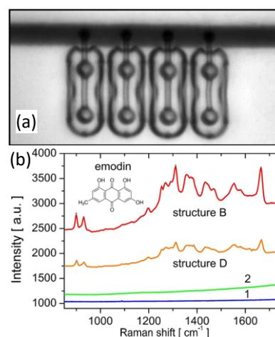
Figure 4: Optical microscopic image of the polymer microtools made with parallel TPP and coated partially with silver NPs (a). SERS spectra of emodin measured with two kinds of structures (red and orange plots) and without the structures (green and blue) (b).
