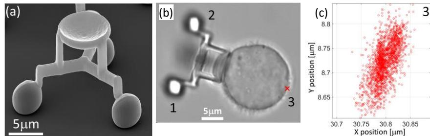
Figure 5: SEM image of the polymer cell manipulator structure (a). Optical microscopic image of a cell attached to a manipulator structure as held by the optical tweezers (b). Fluctuation of point 3 on panel (b) showing the positional stability of the trapped cell (c).
