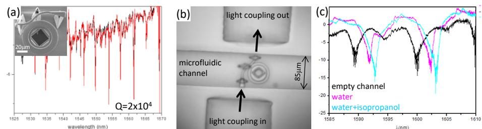
Figure 2: Coupling spectrum of a WG resonator with optimized shape (a); insert: top-view SEM image of the resonator. WG resonator fabricated inside a microfluidic channel (b). Primary results showing the shift of the coupling wavelength when the WG is surrounded with liquid of different refractive indices (c).
