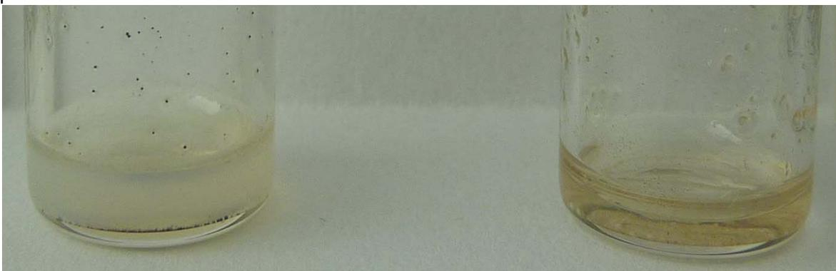
Fig. 3. Photograph made on two ferronematics prepared in the identical procedure, with the same spherical  $Fe_3O_4$  nanoparticles (having a mean diameter of 20nm), in the same volume concentration ( $10^{-4}$ ), however, in different LC matrices: 6CHBT (on the left), and 6CB (on the right). Before taking the photograph, the samples were slightly shaken, so that the FN wets the side-wall for better visibility.
