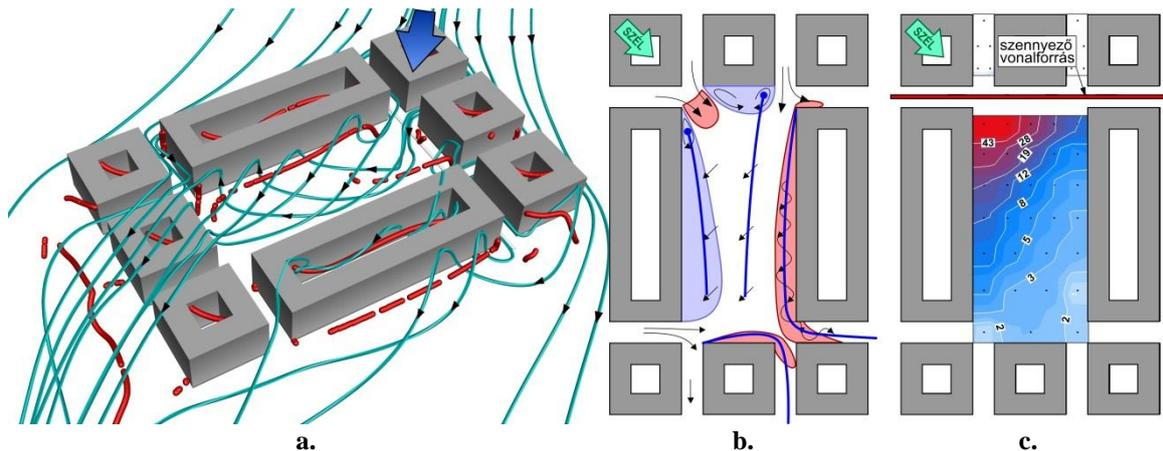
Figure 3. 3D flow features in an urban square at slanted flow direction (thick red lines: vortex cores), b: flow schematics of the square, light blue low speed zone, red: high speed zones thick blue lines: vortex cores. c) pollutant dispersion field in the square.
