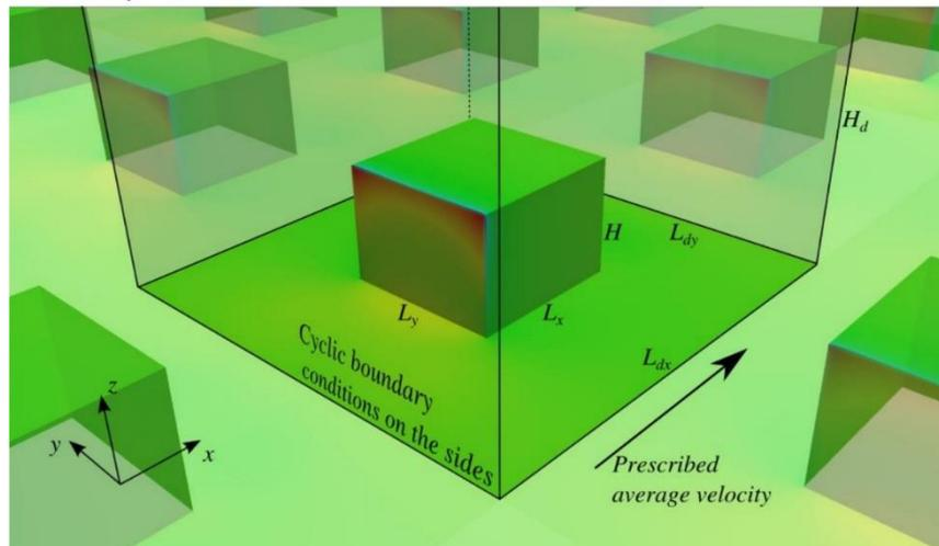
Figure 2. Schematic of the geometrical setup for the series of numerical simulations.
